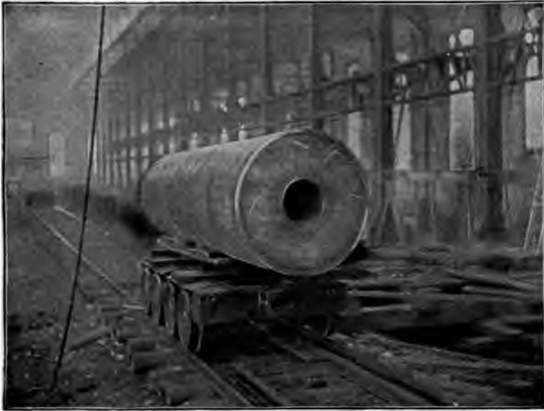
FIG. 231.—INGOT WITH 16-INCH CENTRAL HOLE AS DRILLED.
