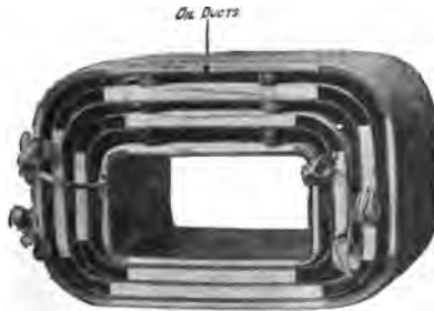
FIG. 152.—Core type coils assembled.
