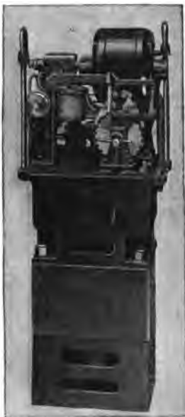
FIG. 218.—View of mechanism and core of pole type induction regulator.
