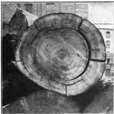
FIG. 27.—Ring Shakes in Chestnut Pole.
