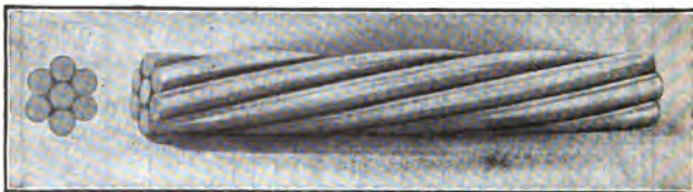
FIG. 83. Seven steel wires twisted into a single strand.
