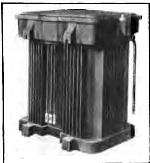
Fig. 159.—Self cooling out-door type transformer, three-phase, 100 kv-a, 2,200/220 volts, 60 cycles.
