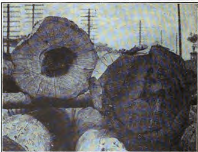
FIG. 22.—Butt Rot in Eastern White Cedar Poles.
