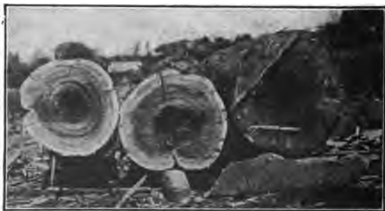
FIG. 20.—Butt Rot in Eastern White Cedar Pole. Right hand section was cut 5 feet from Butt. Middle section was cut 10 feet from Butt. Left hand section shows remainder of the pole.
