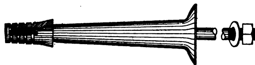
FIG. 102.—Forged pin with separable thimble.
