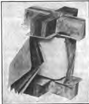
FIG. 150.—Secondary winding assembled on cruciform type transformer core.
