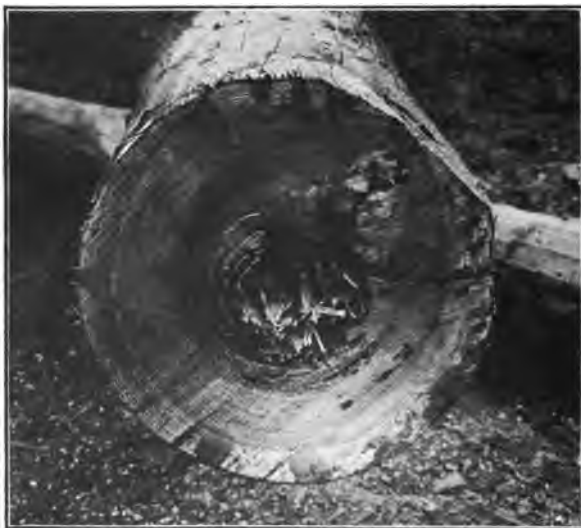
FIG. 33.—Ant Esten Butt in Chestnut Pole.
