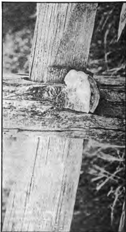
FIG. 343.—Fruiting body on chestnut fence post.
