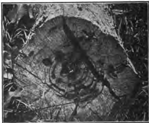
FIG. 28.—Butt Rot and Ring Shakes in Eastern White Cedar Pole.
