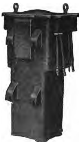
FIG. 217.—Pole type induction regulator showing cast lugs for hanging on transformer hooks.
