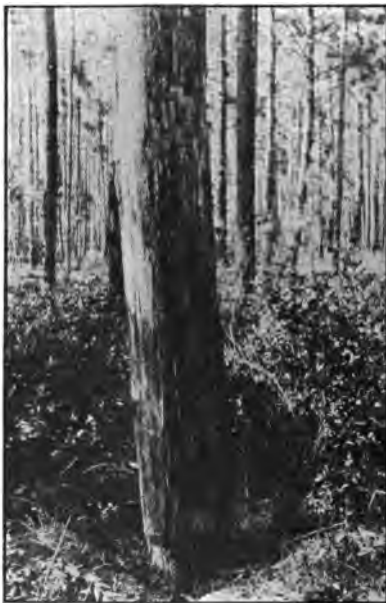
FIG. 351.—Untreated chestnut pole showing falling off of sap-wood.
