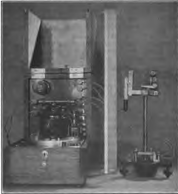
FIG. 1— ABERDEEN CHRONOGRAPH, FALL APPARATUS AND DIRECT-READING VELOCITY SCALE. INSTRUMENTS IN OPERATING POSITION.
