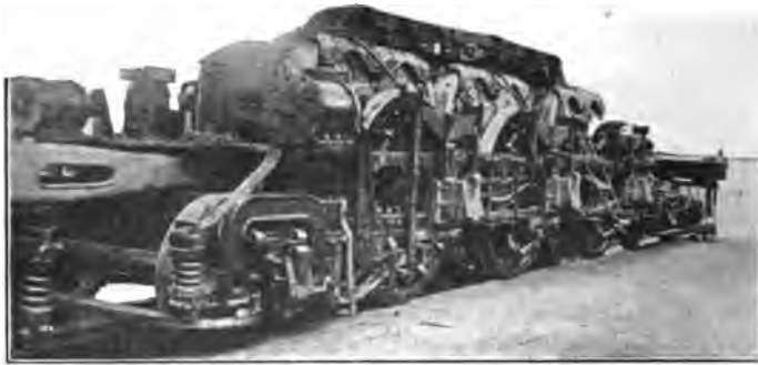
FIG. 3—ONE-HALF LOCOMOTIVE RUNNING GEAR, SHOWING DRIVING MOTORS, COUPLING BAR AND AIR CONDUIT
