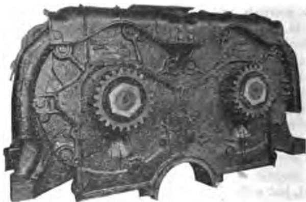
FIG. 4—700-H. P. 1500/3000-VOLT D-C. TWIN ARMATURE MOTOR
