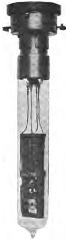
FIG. 7—SMALL RELAY SWITCH OPERATED IN INERT GAS
