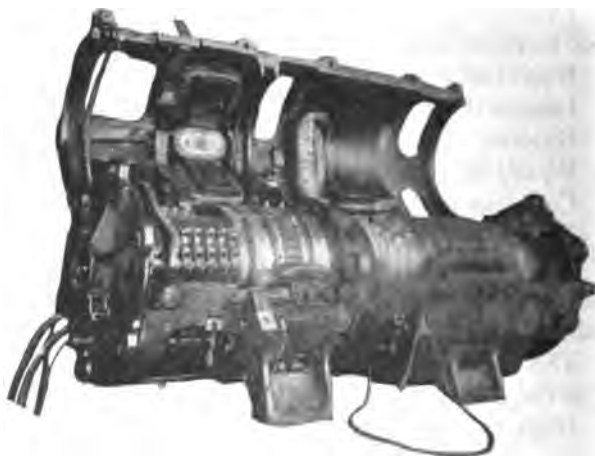
FIG. 16—3000-VOLT-85-VOLT MOTOR-GENERATOR SET—TOP HALF OPENED
