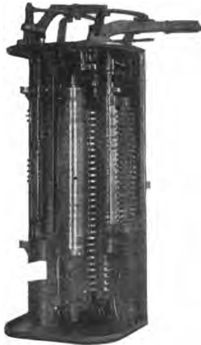
FIG. 9—MASTER CONTROLLER WITH COVER REMOVED, SHOWING DRUMS FOR SPEED CONTROL, REVERSING, MOTOR COMBINATIONS AND REGENERATION
