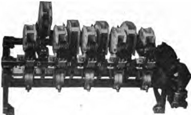
FIG. 13—CAM OPERATED SWITCH GROUP WITH MAGNETIC BLOWOUTS
