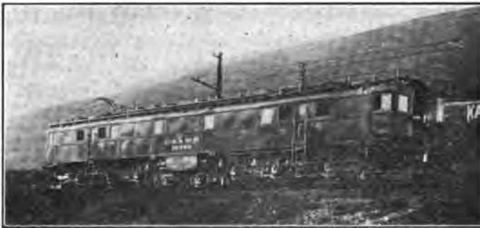
FIG. 1—BALDWIN-WESTINGHOUSE 3000-VOLT D-C. 275-TON PASSENGER LOCOMOTIVE FOR CHICAGO, MILWAUKEE & ST. PAUL RAILWAY Co.
