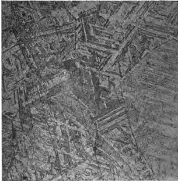
FIG. 20—2 Ni 232 30 PER CENT Ni COOLED TO -70 DEG. CENT. AND REHEATED TO ROOM TEMPERATURE. (100 DIAMETERS)
