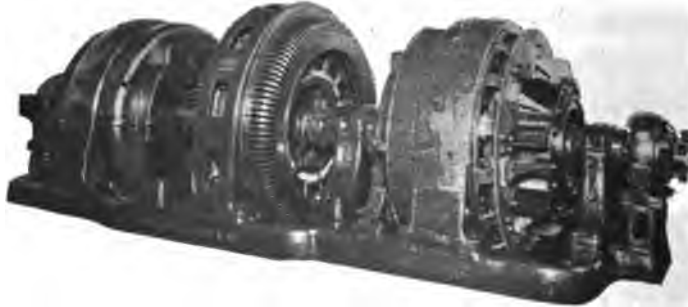
FIG. 9—2000-Kw., 3000-VOLT D-C. SYNCHRONOUS MOTOR-GENERATOR SET EQUIPPED WITH FLASH BARRIERS
