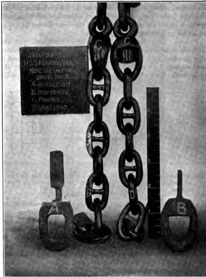
FIG. 1 SECTIONS OF 3 1/2-IN. SHOTS SHOWING POWER-FORGED LINKS AND DROP-FORGED SWIVEL BOXES
