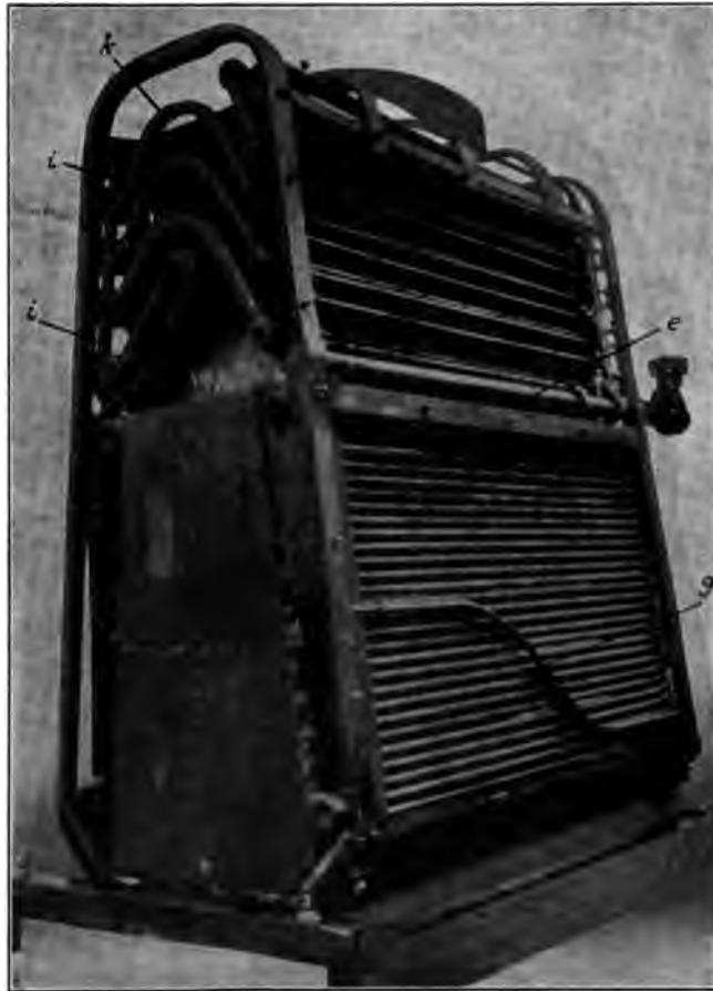
FIG. 2 REAR OF BOILER, CASING REMOVED f Separator, e Main steam pipe, g Separator drain, i Feed pipe, k Trap
