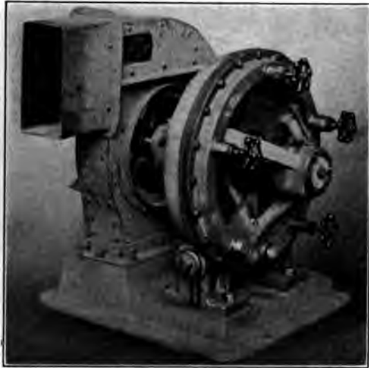
FIG. 18 DIRECT-CONNECTED TURBO-BLOWER EQUIPMENT
