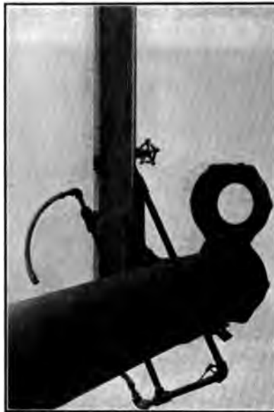
FIG. 3 ORIFICE AT END OF 5-IN. PIPE WITH MANOMETER OR GAGE GLASS CONNECTION
