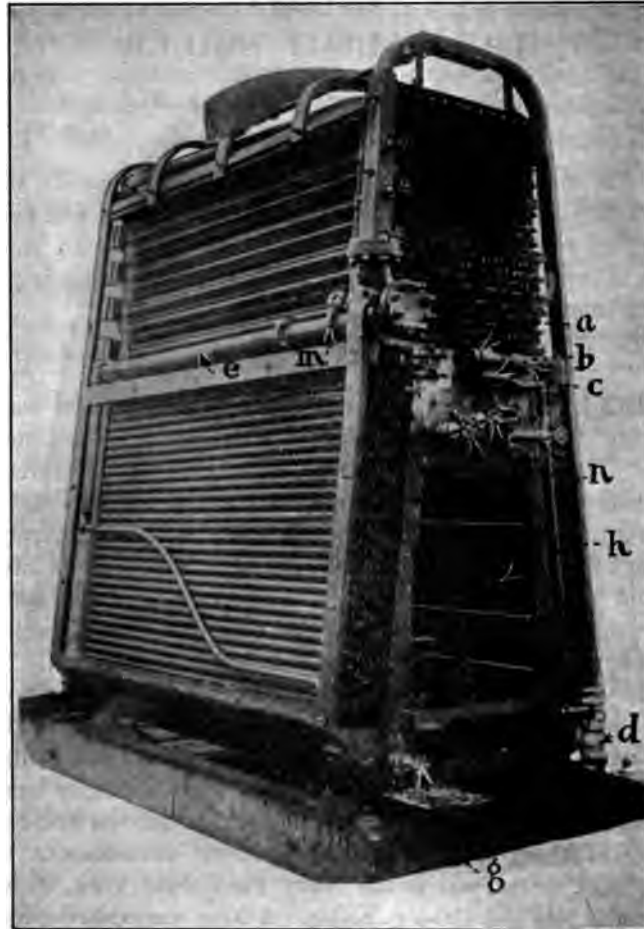
FIG. 1 FRONT OF BOILER, CASING REMOVED
