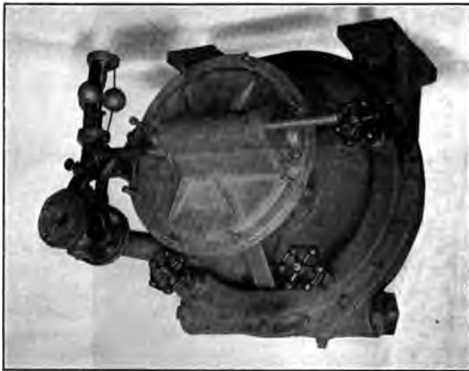
FIG. 19 VARIABLE-SPEED STEAM TURBINE FOR CONTROL OF FUEL-FEEDING MECHANISM, SHOWING SPECIAL GOVERNOR FOR VARYING SPEED OF TURBINE
