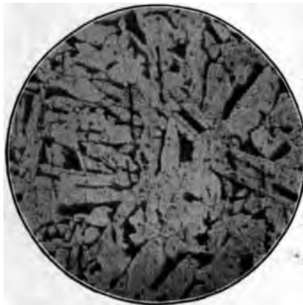
FIG. 4 1 HEAVY PEARLITE STRUCTURE — FROM HEAVILY SHADED AREAS IN FIG. 3
