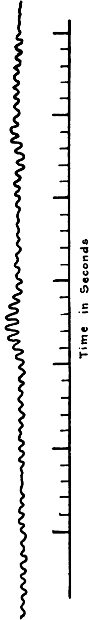
FIG. 4 RECORD NO. 2, TAKEN AT STATION 3 ON SECOND FLOOR. SHOWS LOW AVERAGE AMPLITUDE UNDER SAME CONDITIONS. RECORDS TAKEN AT STATION 2 SHOWED SAME CHARACTERISTICS AS THOSE AT STATION 3
