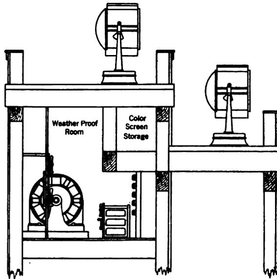
FIG. 5 — CROSS SECTION OF ELECTRIC COLOR SCINTILLATOR
