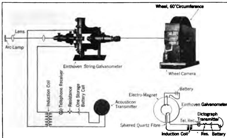
the string corresponded almost exactly to every component of the impressed speech currents, and the resulting speech records should be regarded as being as nearly correct records of speech as can be obtained by any recording instrument.
