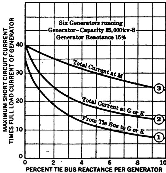
FIG. 4—EFFECT OF TIE BUS REACTANCE SHORT CIRCUIT CURRENT
