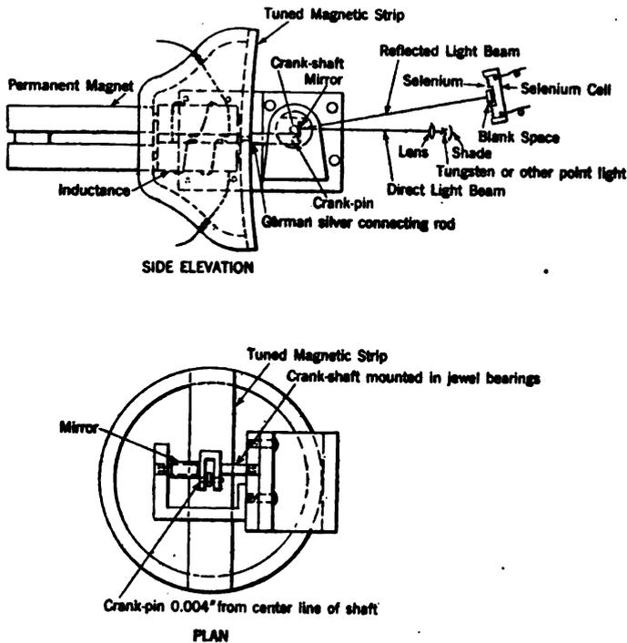
FIG. 2—MECHANICAL ARRANGEMENT OF MIRROR-MOVING MECHANISM OF THE VOICE-OPERATED PHONOGRAPHIC ALPHABET WRITING MACHINE
