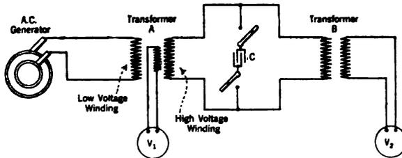
FIG. 6—METHOD OF TESTING THE ACCURACY OF VOLTMETER COIL
