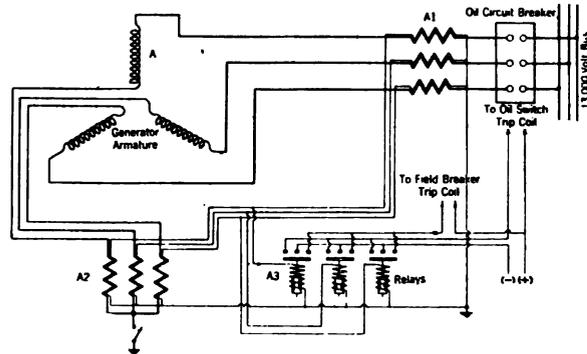
FIG. 1—CONNECTIONS FOR RELAYS ON GENERATORS
