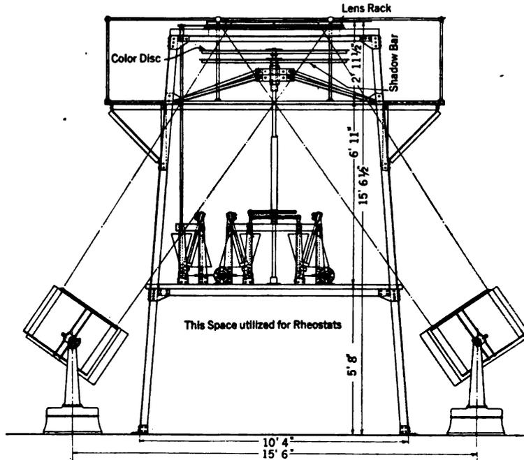
FIG. 11—ELEVATION OF ELECTRIC COLOR KALEIDOSCOPE—PALACE OF HORTICULTURE
