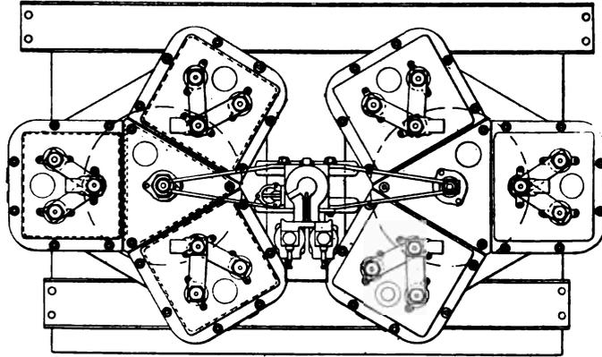
FIG. 4—SKETCH SHOWING HORIZONTAL ARRANGEMENT OF RHEOSTAT TANKS
