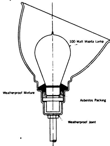
FIG. 19—CROSS SECTION OF ANGULAR WEATHER-PROOFED REFLECTOR
