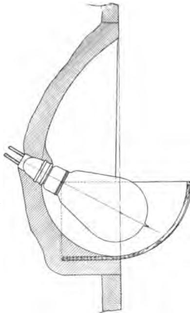
FIG. 21—CROSS SECTION OF COLUMN CUP
