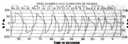
FIG. 8—SPEED CURVE OF REVERSING MOTOR DRIVING MILL
