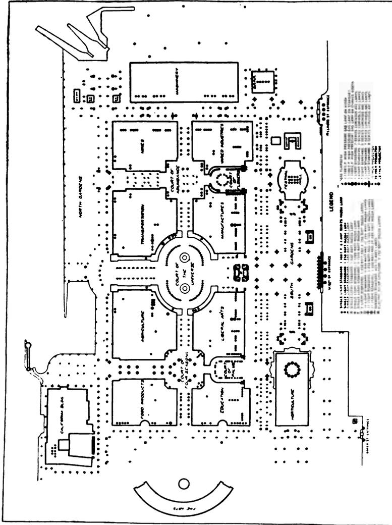
FIG. 25—GROUND AND BUILDING PLAN OF MAIN EXHIBIT PALACES Showing Location of Incandescent and Arc Standards, Gas Emergency Lights and Searchlights
