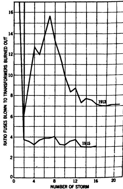
FIG. 15—DIAGRAM SHOWING RATIO OF PRIMARY FUSES BLOWN TO TRANSFORMERS BURNED OUT BY LIGHTNING IN 1913 AND 1915
