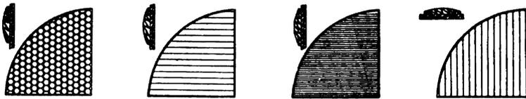
FIG. 13—LENS QUADRANTS FOR ELECTRIC KALEIDOSCOPE—PALACE OF HORTICULTURE
