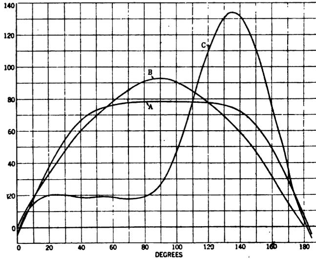
FIG. 5—BUILT-UP WAVES USED IN TESTING CREST VOLTMETER
