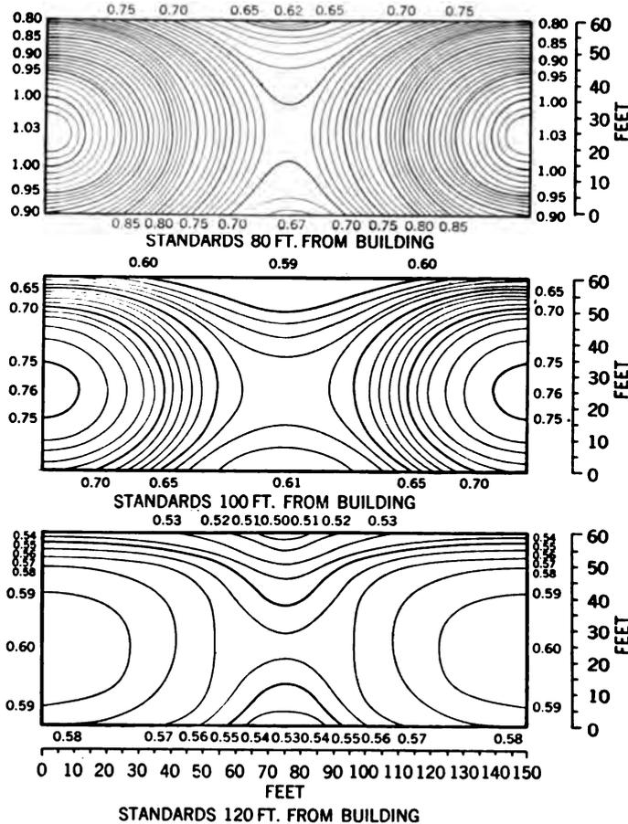
FIG. 7—ILLUMINATION ON EXTERIOR OF BUILDINGS—FIVE LIGHT STANDARDS
