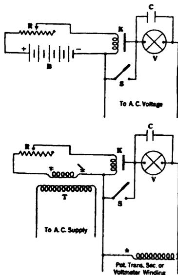
FIG. 4—DIAGRAM OF CONNECTIONS USED IN MEASURING CREST VOLTAGE
