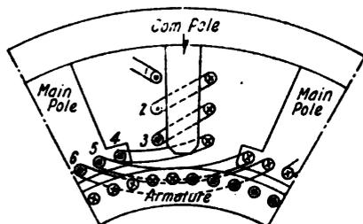
FIG. 11—COMMUTATING POLE AND COMPENSATING WINDING
