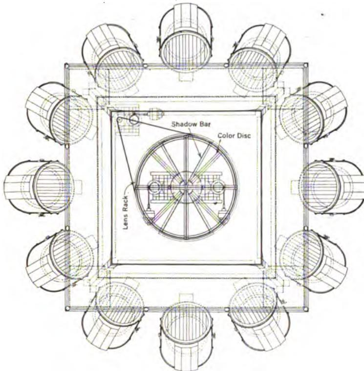
FIG. 10—PLAN VIEW OF ELECTRIC KALEIDOSCOPE—PALACE OF HORTICULTURE
