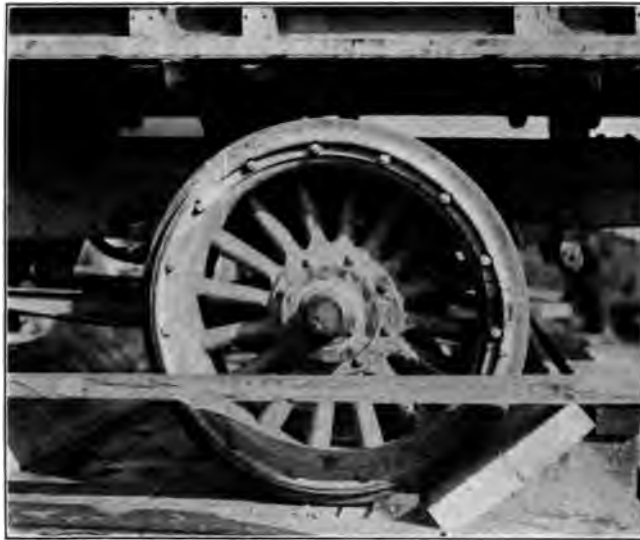
FIG. 7 "CRADLE" IN WHICH TRUCK WAS SURGED TO AND FRO BY ITS OWN POWER
