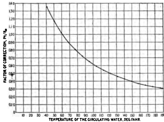
FIG. 3 CURVE OF FACTORS OF CORRECTION FOR CHANGE IN VISCOSITY WITH CHANGE IN TEMPERATURE OF THE CIRCULATING WATER
