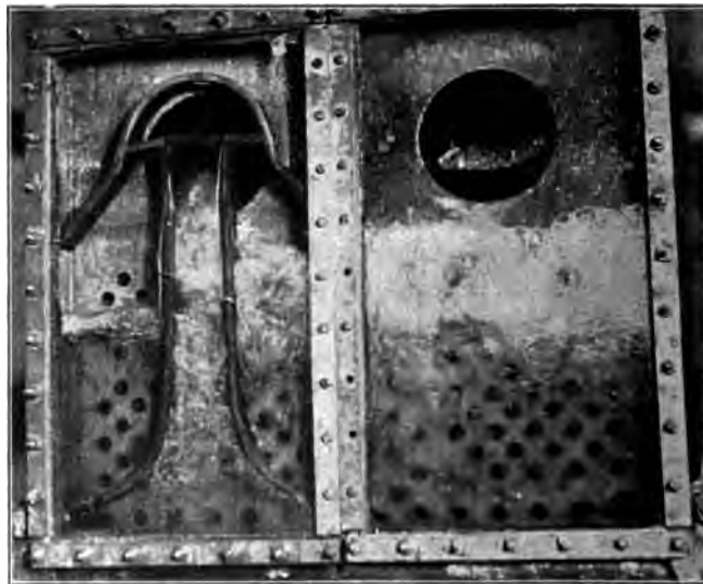
FIG. 12 SHOWING FRONT HEADERS; LOAD 85 PER CENT; SETTING AS IN FIG. 8b; WATER LEVEL BELOW NORMAL
