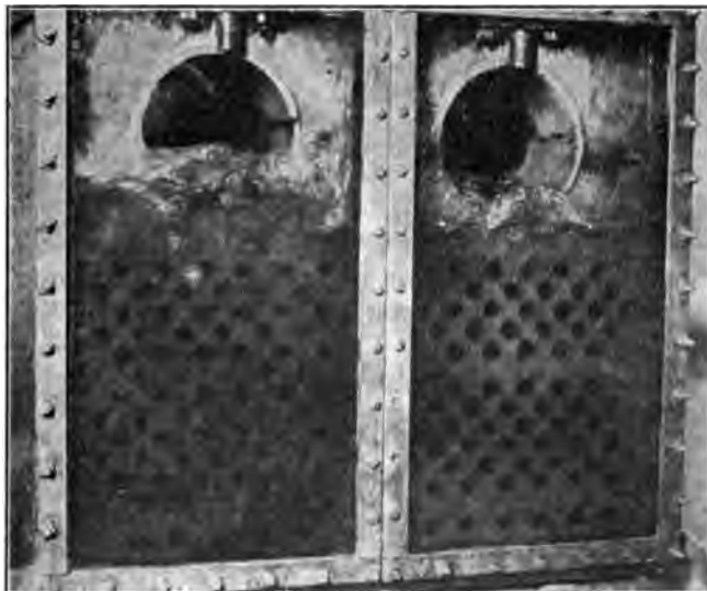
REAR HEADERS CORRESPONDING TO DESIGN OF FIG. 7F AT THE FRONT OF THE LEFT HAND BOILER, AND THE DESIGN OF 7C AT THE FRONT OF THE RIGHT HAND BOILER; LOAD 300 PER CENT; SETTING AS IN FIG. 8b
