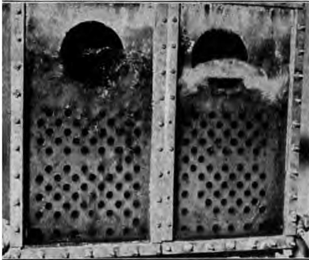
REAR HEADERS CORRESPONDING TO HEADERS OF FIG. 19 IN FRONT; LOAD 450 PER CENT; SETTING AS IN FIG. 8a
