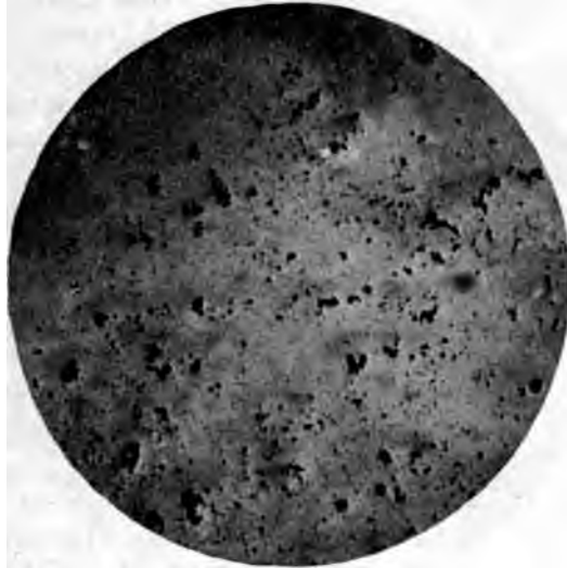
FIG. 12 DISPERSION OF CEMENT PARTICLES BY ALCOHOL
