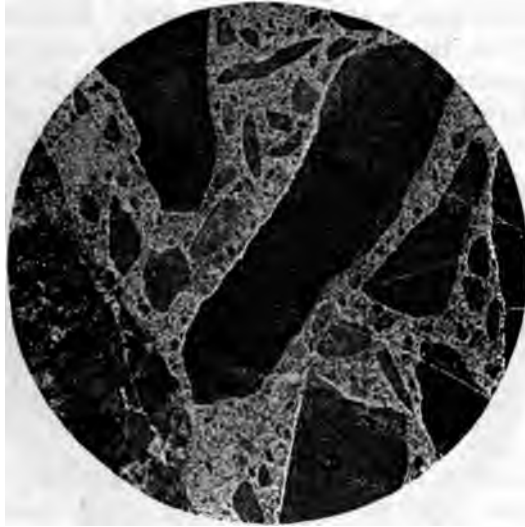
FIG. 3 SECTIONED CONCRETE SPECIMEN, MAGNIFIED 2 DIAM.
