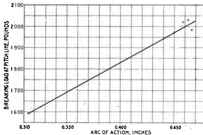
FIG. 4 RELATION OF BREAKING LOAD TO ARC OF ACTION: FELLOWS 20-DEG. INVOLUTE AT 500 FT. PER MIN. PITCH SPEED
