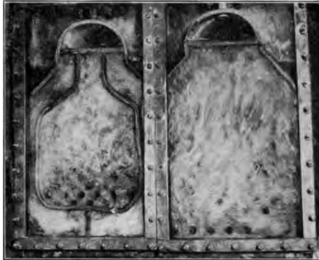
IG. 17 SHOWING FRONT HEADERS; LOAD 500 PER CENT; SETTING AS IN FIG. 8a
