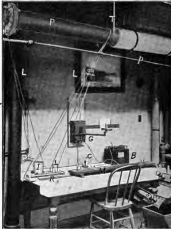
FIG. 3 APPARATUS FOR INVESTIGATING TEMPERATURE GRADIENT IN THE WALL OF A STEAM PIPE
