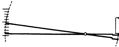
FIG. 3 LEVER EXTENSOMETER FOR MEASURING DEFORMATION
