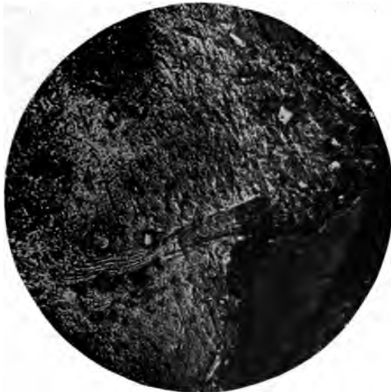
FIG. 13 "SHEAR PLANES" IN CEMENT MATRIX
