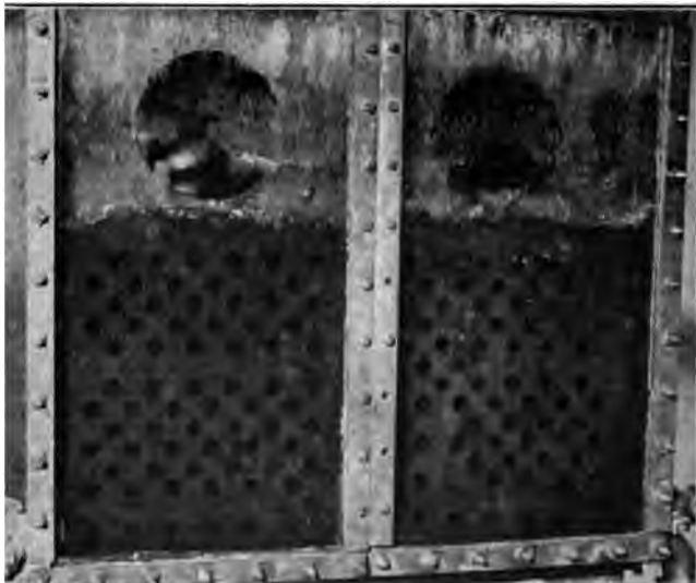
REAR HEADERS CORRESPONDING TO DESIGNS OF FIG. 19 IN FRONT; LOAD 85 PER CENT; SETTING AS IN FIG. 8a
