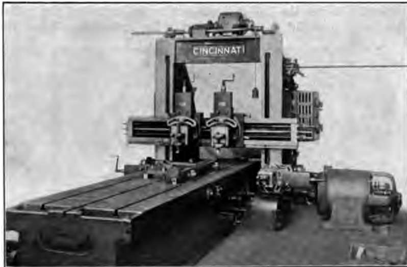
FIG. 18 48-IN. CINCINNATI PLANER DRIVEN BY 20 H.P., 250/1000 R.P.M., 230-VOLT MOTOR
