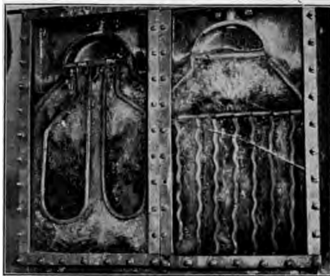
FIG. 19 SHOWING FRONT HEADERS; LOAD 450 PER CENT; SETTING AS IN FIG. 8a
