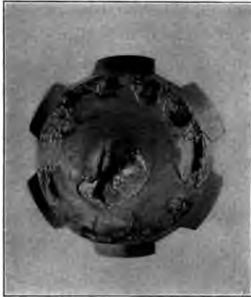
FIG. 3 CHARACTERISTIC FRACTURE SHAFT TURNED DOWN
