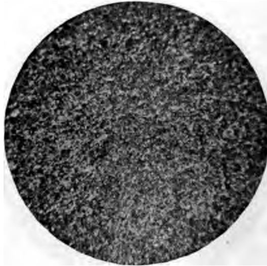
FIG. 7 DRY CEMENT, MAGNIFIED 20 DIAM.
