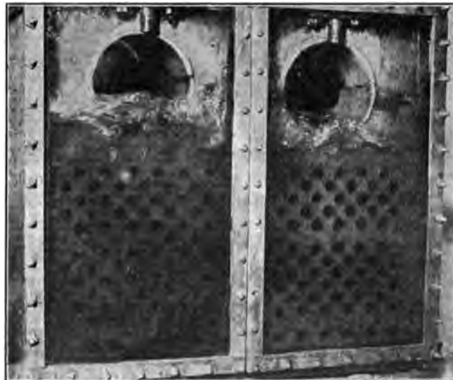
FIG. 26 REAR HEADERS CORRESPONDING TO DESIGN OF FIG. 7F AT THE FRONT OF THE LEFT HAND BOILER, AND THE DESIGN OF 7C AT THE FRONT OF THE RIGHT HAND BOILER; LOAD 300 PER CENT; SETTING AS IN FIG. 8b
