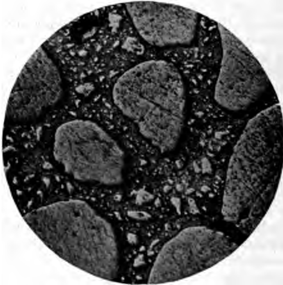
FIG. 1 MICRO-PHOTOGRAPH OF 1:3 MORTAR
