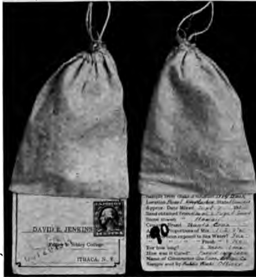
FIG. 9 METHOD USED IN COLLECTING SAMPLES OF FIELD CONCRETE
