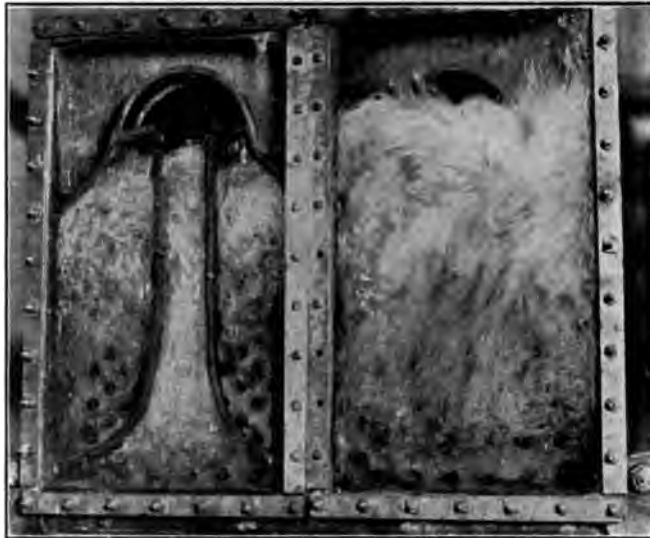
FIG. 13 SHOWING FRONT HEADERS; LOAD 275 PER CENT; SETTING AS IN FIG. 8b
