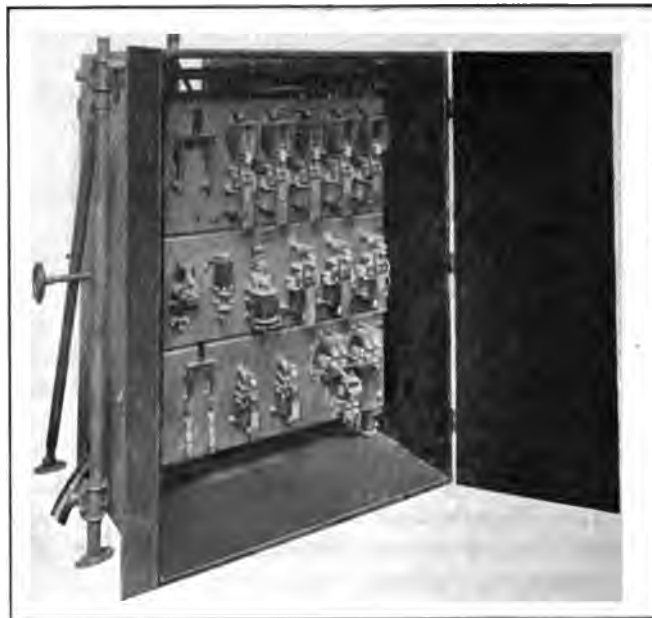
FIG. 13 CONTROL PANEL FOR 50 H.P. AND 7\frac{1}{2} H.P. COMBINATION BORING MILL MOTOR
