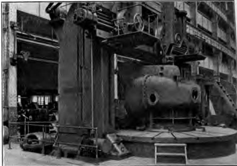
FIG. 12 WILLIAM SELLERS 18 FT. BORING MILL OPERATED WITH 7\frac{1}{2} AND 50 H.P. MOTORS CONTROLLED BY PANEL. A IS RAPID TRANSVERSE AND FEED CONTROL STATION, B IS MOTOR PANEL AND C IS MAIN MOTOR CONTROL STATION
