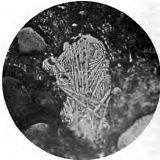
FIG. 2 MICRO-PHOTOGRAPH OF 34-YR. OLD CONCRETE
