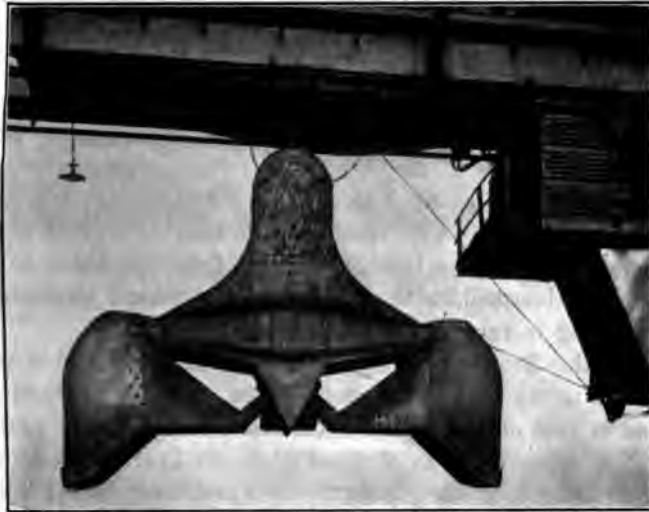
FIG. 33 HEYL AND PATTERSON MAN TROLLEY AND 12-TON UNLOADING CLAMSHELL ON NORTH WESTERN FUEL COMPANY'S No. 5 BRIDGE
