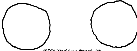
15" Chilled Iron Wheel with Flat Tread, 200,000 lb. load on standard A.S.C.E. rail Area of depression in rail 130 sq.in.
