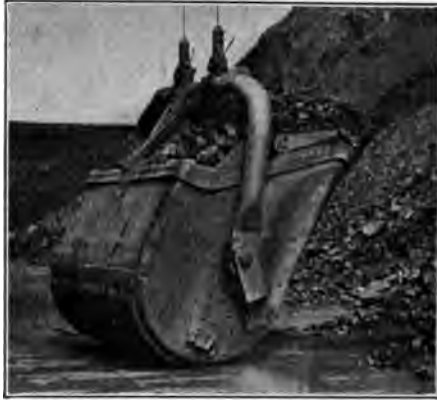
FIG. 30 BROWN 4-TON SHOVEL BUCKET ON NORTH WESTERN FUEL COMPANY'S SUPERIOR DOCK NO. 1
