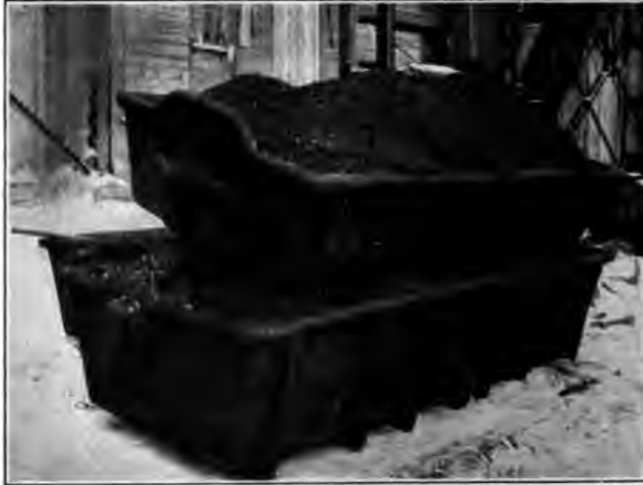
FIG. 8 CUTTINGS PRODUCED BY MILLING
