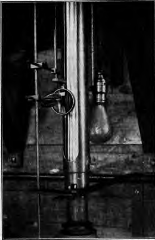
FIG. 7 HOOK-GAGE COLUMN, SHOWING MAGNIFYING GLASS AND MIRROR
