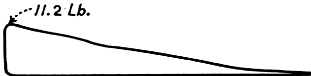
FIG. 2 DIAGRAM SHOWING VARIATION OF PRESSURE DURING THE DISCHARGE STROKE OF AN AIR COMPRESSOR
