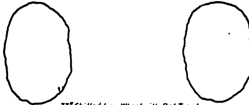
33" Chilled Iron Wheel with flat Tread, 200,000 lb. load on standard A.S.C.E. rail. Area of depression in rail 1.35 sq.in.
