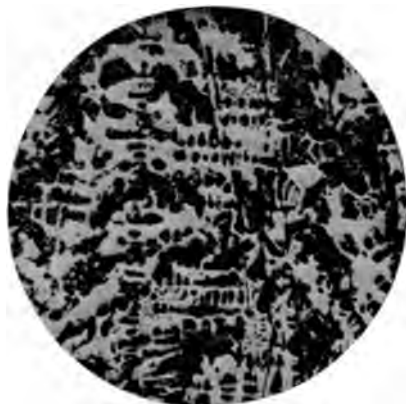
FIG. 40 BAD WHEEL. \frac{1}{4} IN. FROM CHILL
