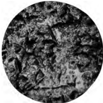
FIG. 42 BAD WHEEL. BACK OF TREAD MAGNIFIED 75 DIAMETERS
