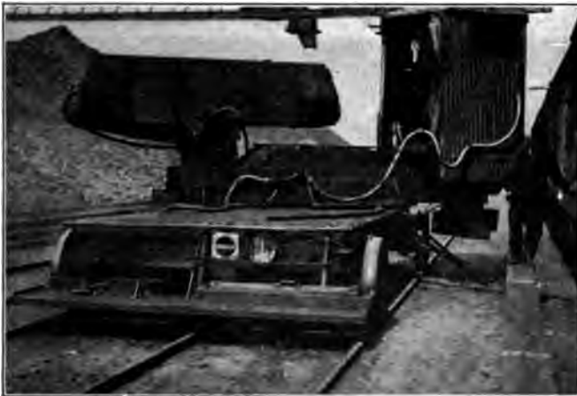
FIG. 37 CHRISTY BOX CAR LOADER COMPANY'S ELECTRIC SWIVELING CONVEYOR LOADER, INSTALLED ON NORTH WESTERN FUEL COMPANY'S DOCK No. 1, SUPERIOR, 1913
