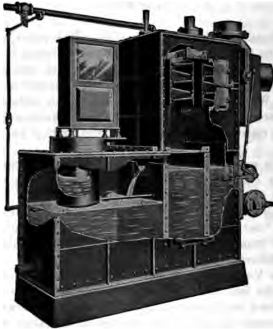
FIG. 1 V-NOTCH METER COMBINED WITH FEEDWATER HEATER
