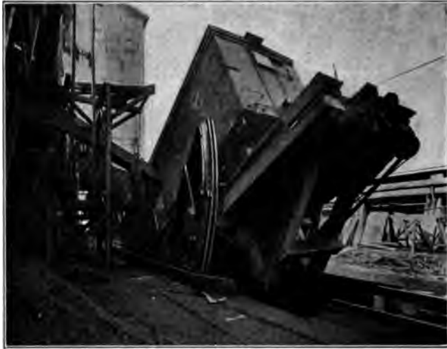
FIG. 38 SMITH TILTING BOX CAR LOADER, BUILT BY THE DODGE COAL STORAGE COMPANY
