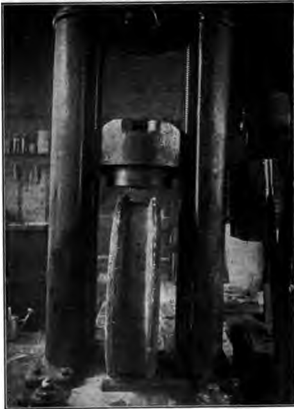
FIG. 12 300,000-LB. RIEHLE TESTING MACHINE SHOWING POSITIONS OF WHEEL AND TOGGLE WHEN TESTING STRENGTH OF FLANGES
