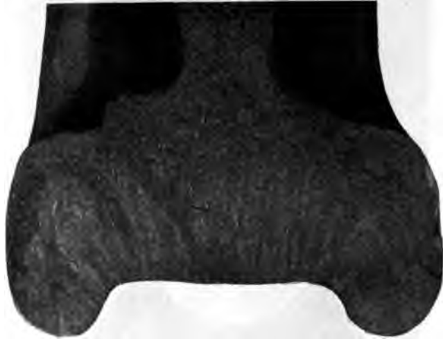
FIG. 14 SECTION OF A DOUBLE FLANGE CRANE WHEEL SHOWING CHILLED IRON IN TREAD
