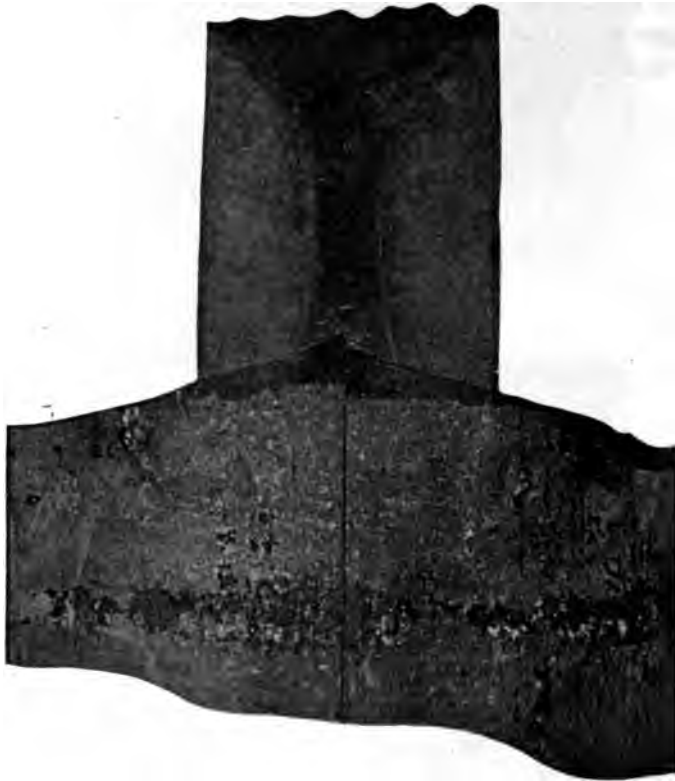
FIG. 11 PIECE OF RAIL BROKEN UNDER THE DROP PRESS
