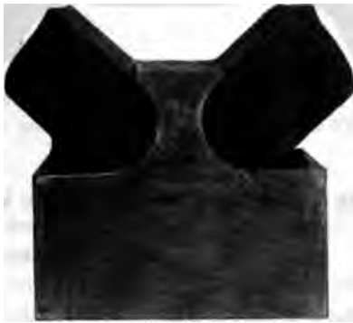
FIG. 13 TOGGLES USED IN TESTING STRENGTH OF FLANGES
