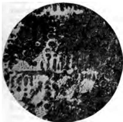
FIG. 38 GOOD WHEEL. CENTER OF TREAD
