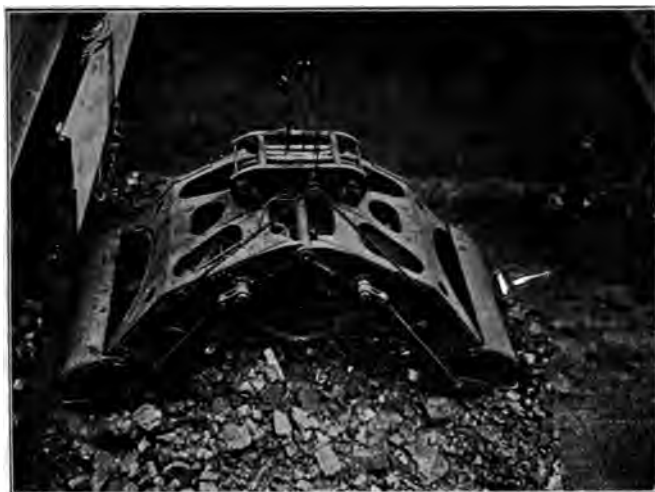
FIG. 34 HEYL AND PATTERSON 4-TON CLEAN-UP CLAM, INSTALLED ON NORTH WESTERN FUEL COMPANY'S DOCK No. 2, IN 1912
