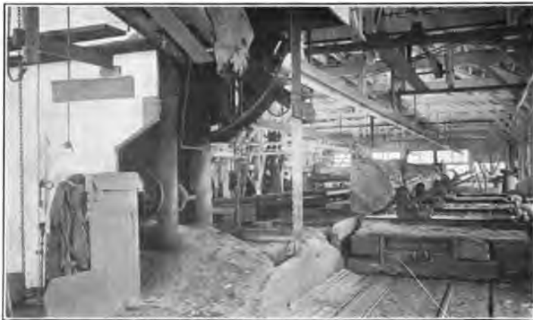
[WHITNEY] FIG. 15—TEN-FOOT BAND HEADSAW AND LOG CARRIAGE AT END OF TRAVEL. BOARD WHICH HAS JUST BEEN CUT IS LYING ON LIVE ROLLS
