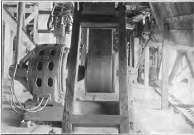
[WHITNEY] FIG. 19—250-H. P. SQUIRREL CAGE MOTOR DRIVING DOUBLE 66-IN. CIRCULAR HEADSAW IN PACIFIC COAST MILL
