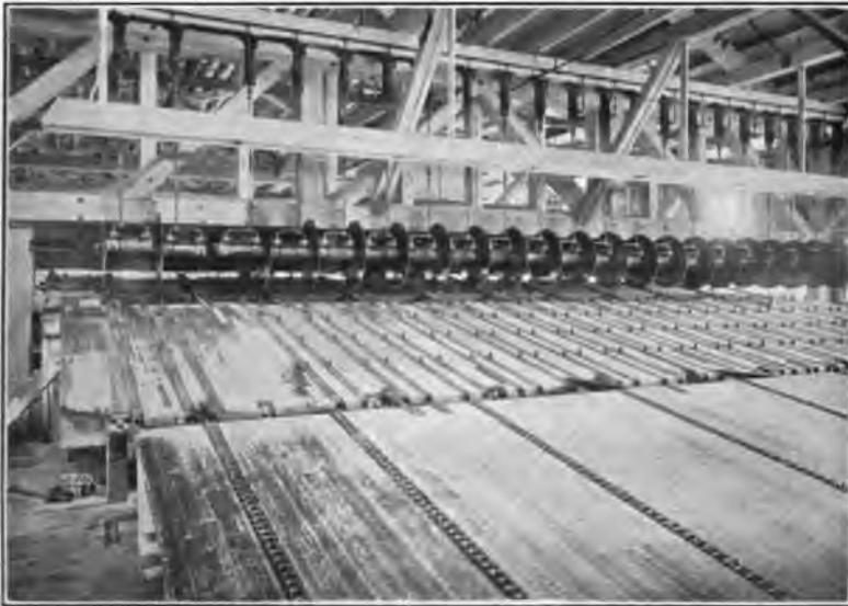
FIG. 25—FRONT OF 40-FT. TRIMMER REQUIRING A 50-H. P. MOTOR
