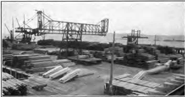
[WHITNEY] FIG. 42—FOUR-TON MONORAIL LUMBER-HANDLING CANTILEVER CRANE, 106 FT. TROLLEY TRAVEL, HAMMOND LUMBER COMPANY, ASTORIA, ORE.
