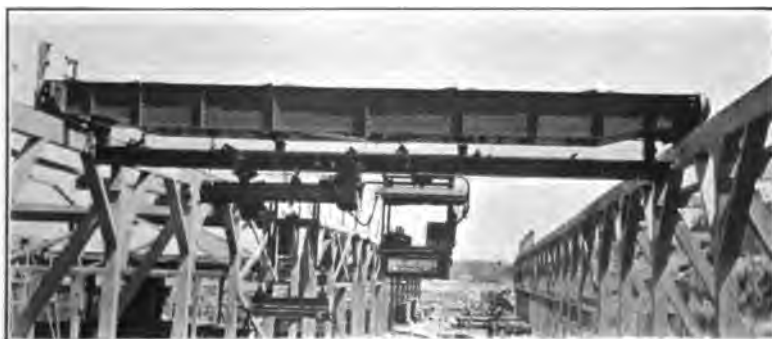
[WHITNEY] FIG. 39—MONORAIL CAR AND TRANSFER CRANE FOR SPOTTING CAR AT DIFFERENT SECTIONS OF SORTING TABLE
