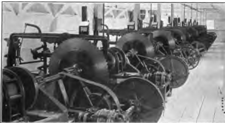
FIG. 52—INTERIOR OF SHINGLE MILL USING ELECTRIC DRIVE. THE COMPACT MACHINES AND ABSENCE OF TRANSMISSION BELTING IS IN MARKED CONTRAST TO THE CROWDED APPEARANCE OF BELT-DRIVEN MILLS
