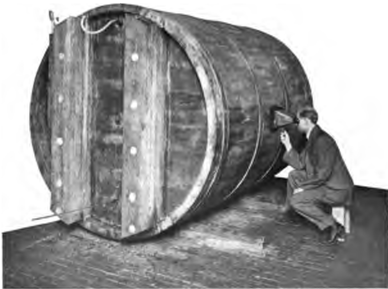
FIG. 1—CASK FOR STUDY OF VARIATION OF SPARK-OVER AND CORONA VOLTAGE WITH AIR DENSITY OR ALTITUDE
