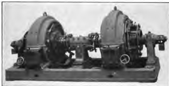
FIG. 10—Two 750-VOLT, 60-CYCLE SYNCHRONOUS CONVERTERS CONNECTED IN SERIES
