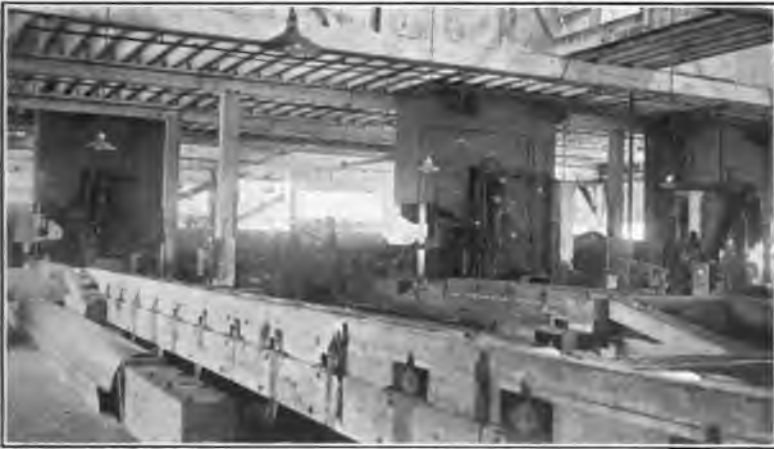
FIG. 17—MILL FLOOR, SHOWING THREE NINE-FOOT BAND HEADSAWS
