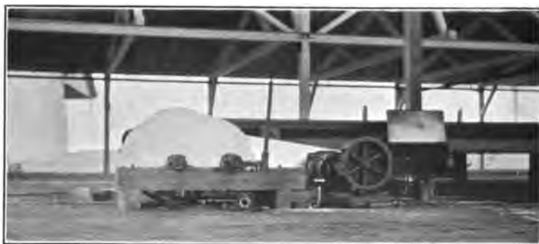
FIG. 48—SORTING TABLE DRIVE IN PLANING MILL, WITH BACK-GEARED MOTOR
