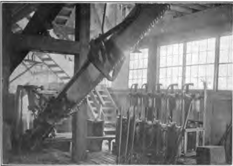
FIG. 11—LOG SAW ON LOG DECK IN MILL. CONTROL FOR LOG HAUL AND CONVEYER CHAINS SHOWN AT RIGHT
