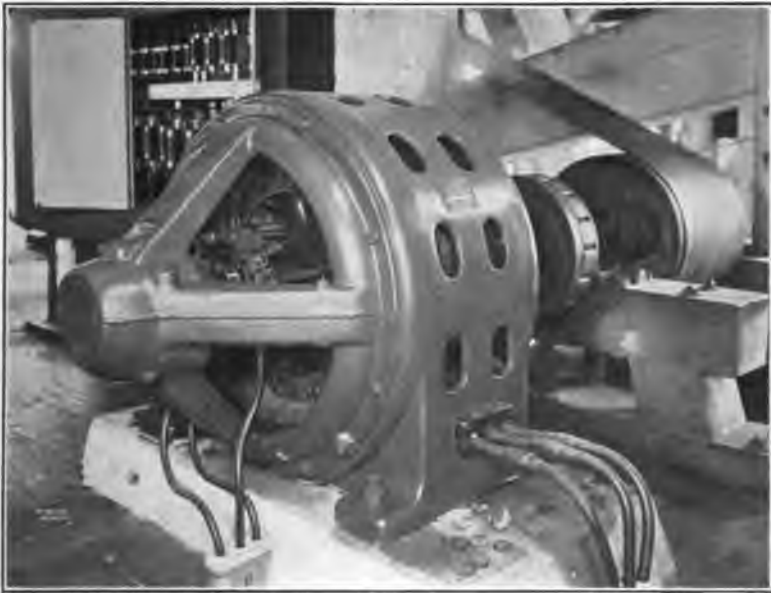
FIG. 18—300-H. P. MOTOR DRIVING 10-FT. BAND SAW IN PACIFIC COAST MILL
