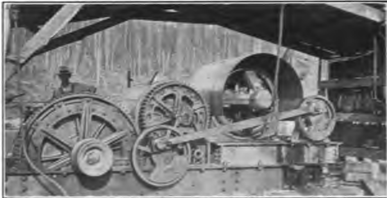
FIG. 3—FIRST TRIAL OUTFIT, USING STANDARD MOTOR EQUIPMENT This outfit operated successfully under varying conditions for a period of three months, to obtain data for later applications.
