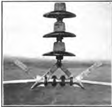
FIG. 4—150,000-VOLT SUSPENSION INSULATOR, SHOWING ARCING RODS.
