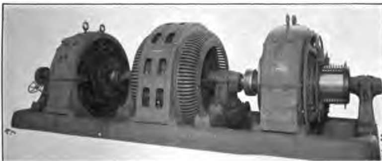
FIG. 11—2400-VOLT MOTOR-GENERATOR SET CONSISTING OF ONE 1450- Kv.A., 2300-VOLT 60-CYCLE SYNCHRONOUS MOTOR AND TWO 500-Kw., 1200-VOLT, D-C. GENERATORS IN SERIES
