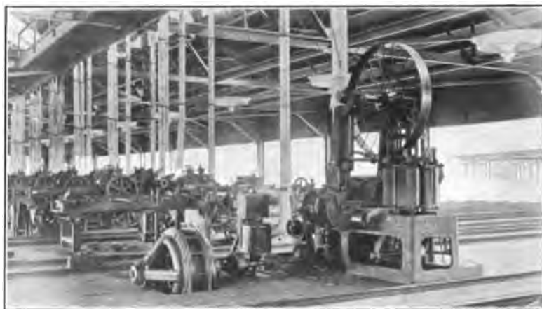
FIG. 28—BAND RE-SAW WITH DIRECT-CONNECTED MOTOR [WHITNEY]
