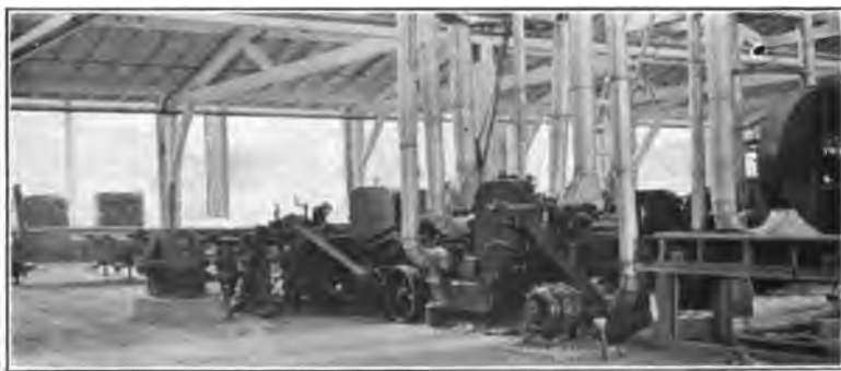
[WHITNEY] FIG. 44—MATCHER WITH 50-H P. MAIN MOTOR AND 15-H.P. PROFILE ATTACHMENT MOTOR
