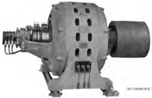
FIG. 11—THREE-PHASE COMPENSATED GENERATOR.
