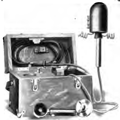
FIG. 28—PORTABLE TELEPHONE STATION, INCLUDING TRANSMITTER, RECEIVER, MAGNETO AND CONNECTION TO LINE BY MEANS OF A "POLE JACK."
