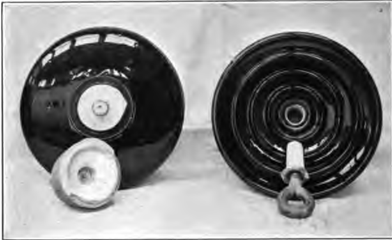
FIG. 11 d —TYPE E—FAILURE OCCURRED AT 7500 LB.
