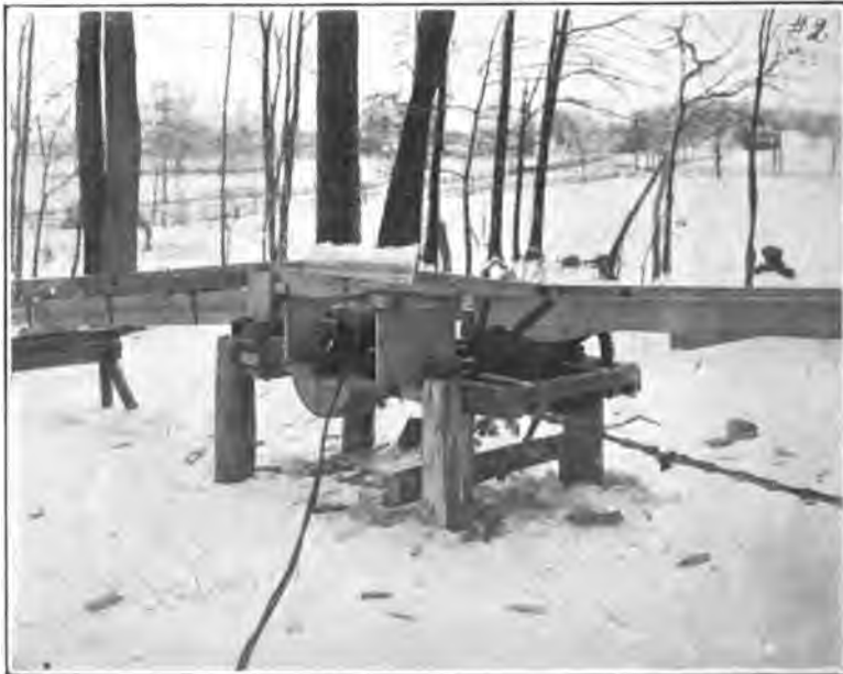
FIG. 22—A 2½-H.P. MOTOR, CONNECTED BY 200 FT. OF FLEXIBLE [BATES] CABLE WITH THE ELECTRICAL SUPPLY OF THE NEAREST BUILDING, DRIVES THIS ICE HARVESTER.
