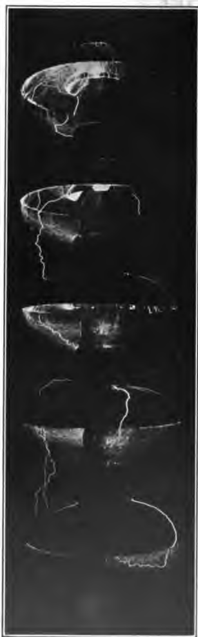
FIG. 10c—SAME AS PRECEDING TEST (b) EXCEPT VOLTAGE RAISED TO 300 KV.
