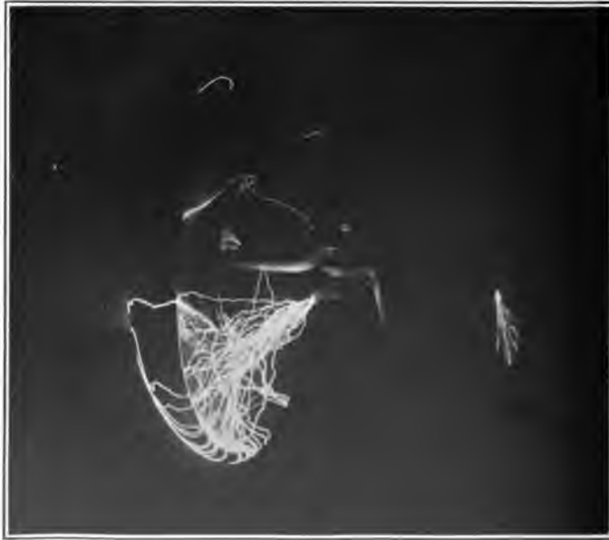
[SOTHMAN] FIG. 9a—TYPE D—ONE SECTION AT 117 KV. Note discharge localized at point of hook.
