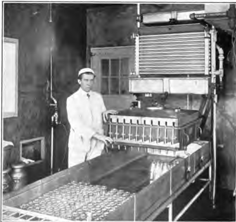
[BATES] FIG. 13—IN A DAIRY OR CREAMERY PLANT ELECTRIC FIXTURES MUST BE WATERTIGHT.
