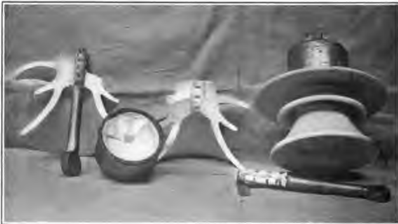
FIG. 11 e —TYPE F—AVERAGE BREAKING LOAD 6900 LB.
