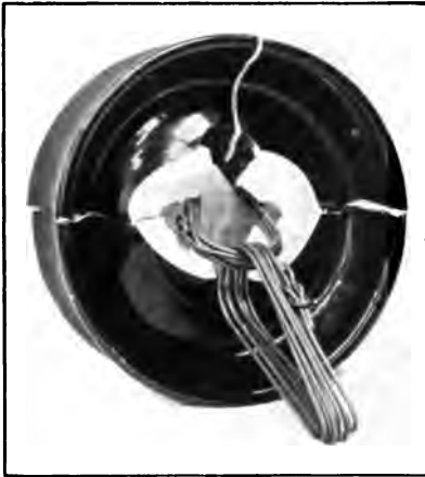
FIG. 11a—TYPE B—FRACTURE OCCURRED AT 8000 LB.
