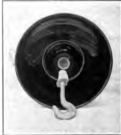
FIG. 11c—TYPE D—HOOK PULLED OUT AT 9000 LB.
