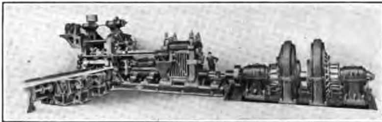
FIG. 9.—Universal plate mill at the Illinois Steel Company's plant, showing the motor drive
