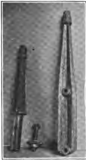
Malleable cast iron pins. Cross-arm pin fits 1\frac{1}{2} -in. hole in old crossarms. T-headed bolt slips into a seat on a shoulder cast on inside of shank at bottom, and is tightened up under cross-arm. Weights 3\frac{1}{2} and 7 lb. Ultimate strength 1800 lb. at line wire. (60,000 volts)
