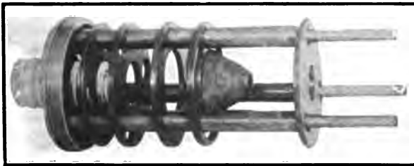
FIG. 17.—Oil diverter of H-3 oil circuit breaker used in test No. 61
