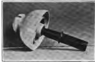
Porcelain insulator and iron pin used on 30,000-volt line
