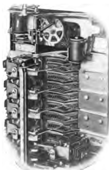
FIG. 4—Close view of line switch unit
