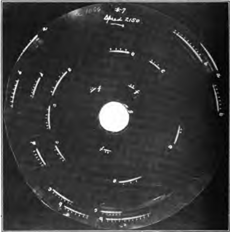
FIG. 4.—Record from revolving film duration apparatus showing six multiple strokes marked a , b , c , d , e , and f . The small dots at the side of most of the exposures are ink marks to emphasize the markings of the natural frequency of the discharge for fear they might not show up in the usual process of reproduction. This record is unusual in the number of multiple strokes
