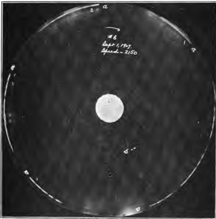
FIG. 3.—Record from revolving film duration apparatus. This shows one multiple discharge consisting of eight single discharges marked (a) and one single discharge marked (b)
