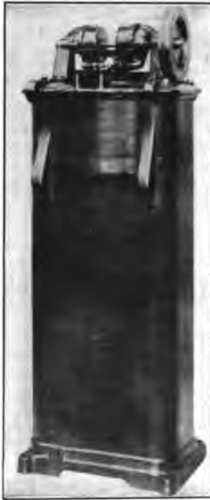
FIG. 7.—Automatically operated switch type of regulator.
