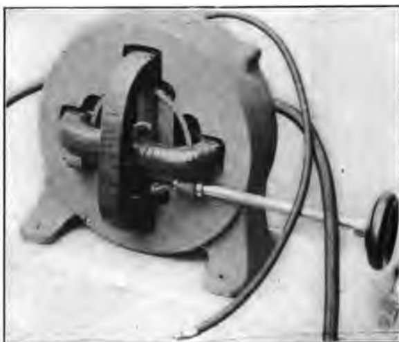
FIG. 3.—Induction regulator with movable core.
