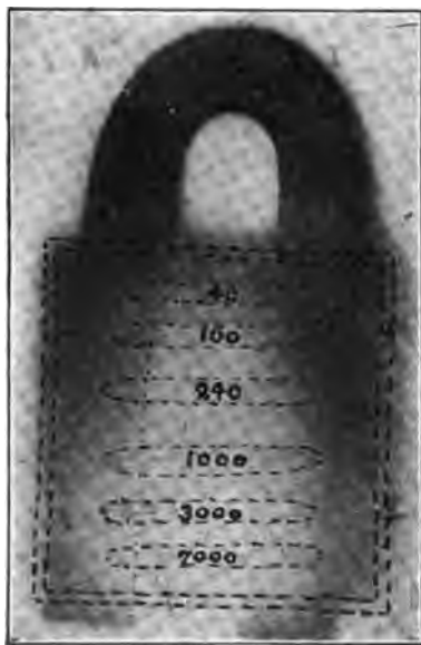
FIG. 8.—Radiograph showing Degrees of Penetration of a thick sheet of Lead and a Steel Magnet by Tubes of Radium of Different Radioactivities.
