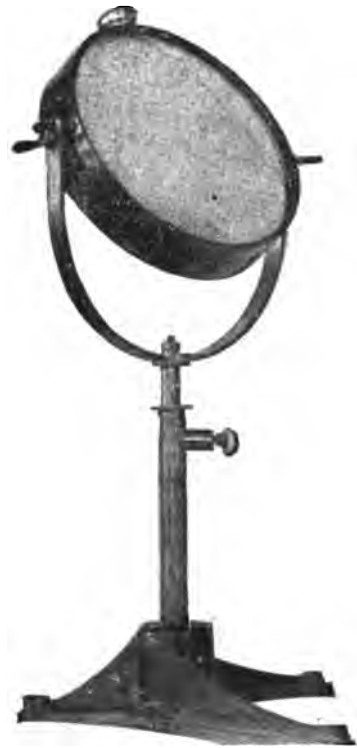
FIG. 34 —Finsen's Original Blue Lens for Use with Sunlight.
