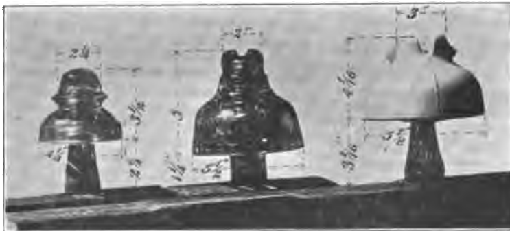
FIG. 5.—Insulators used in High-Tension Tests at Telluride.
