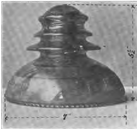
FIG. 16.—Insulator used at Provo for 40,000 volts.
