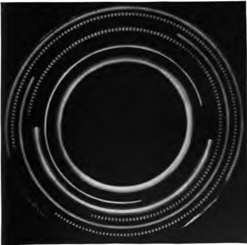
FIG. 15. Chronograph Records of the Alternating Current, under varying conditions of circuit and speed of plate.
