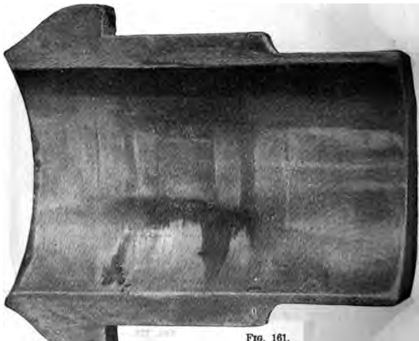
FIG. 161. Brass A.—Irregular dark areas show oil burnt by heat due to action of emery.
