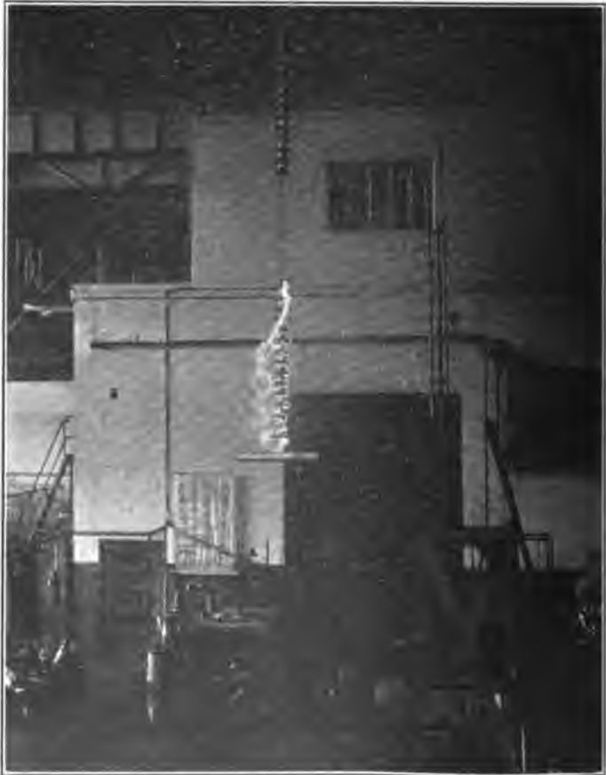
FIG. 23—WET ARC-OVER—CITY WATER—THREE-LINE UNITS WITH INTERNAL SHIELDS TO INCREASE ELECTROSTATIC CAPACITY
