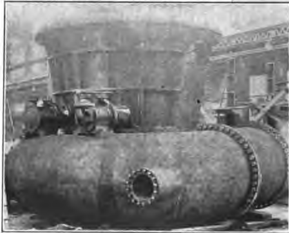
FIG. 19—11,000-H. P. VERTICAL-SHAFT TURBINE Single-runner, cast iron, spiral-cased type, 360-rev. per min., 258-ft. head. Supporting barrel ready for generator.
