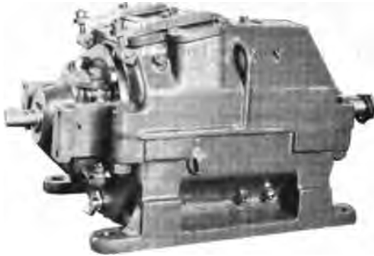
FIG. 3—MARINE D-C. MOTOR—ENCLOSED, FOR OPERATING DECK MACHINERY
