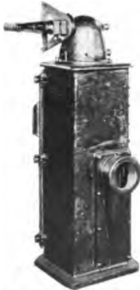
FIG. 4—MARINE CONTROLLER FOR DECK MACHINERY MOTORS
