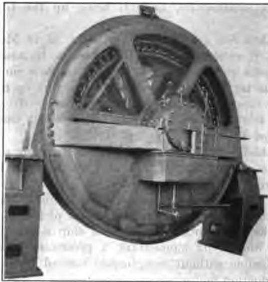
FIG. 5—THRUST BEARING END OF 60-POLE, 3000-H. P., 50-CYCLE, 100-REV. PER MIN., SYNCHRONOUS MOTOR FOR SHIP PROPULSION
