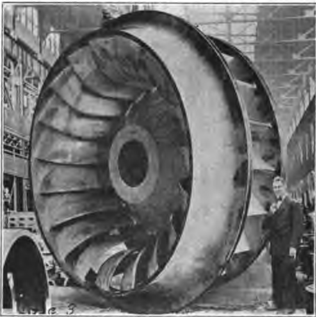
FIG. 3—SHOP VIEW OF 125-IN. CAST IRON RUNNER FOR THE LARGEST COMBINED HYDROELECTRIC UNIT IN THE WORLD
