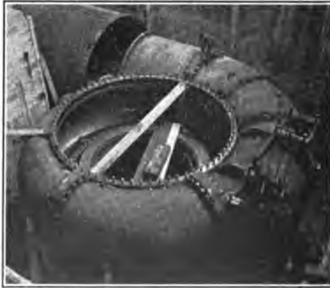
FIG. 19—ONE OF THE CAST IRON TURBINE CASES
