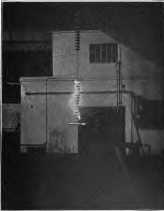
FIG. 22—WET ARC-OVER—CITY WATER—THREE-LINE UNITS WITH INTERNAL SHIELDS TO INCREASE ELECTROSTATIC CAPACITY
