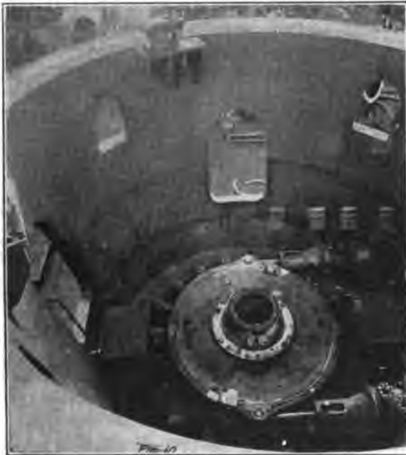
FIG. 10—INSIDE VIEW OF SINGLE VERTICAL TURBINE WITH STEEL PLATE SPIRAL CASING AND CAST IRON SUPPORTING BARREL FOR GENERATOR
