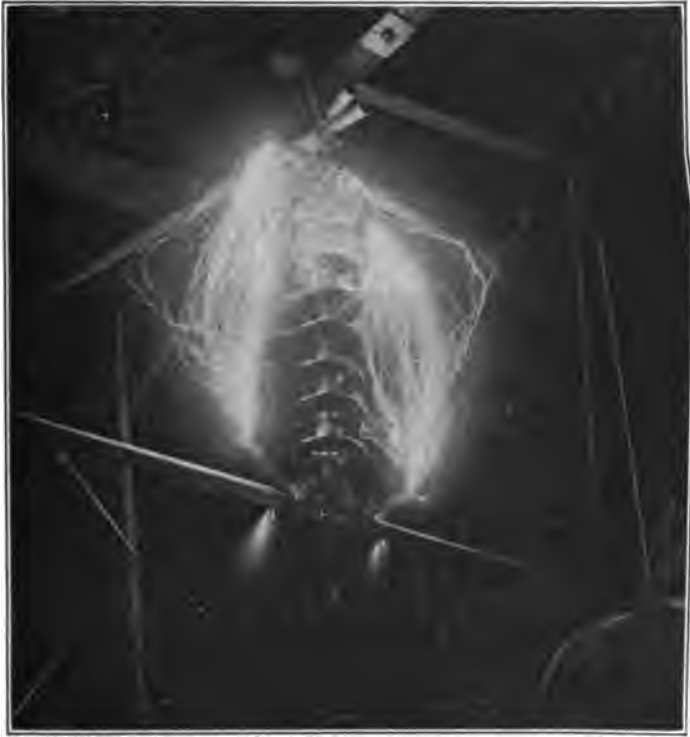
FIG. 28—NINE UNITS—30 FLASH-OVERS—10 CLEAR AND 20 CASCADE
