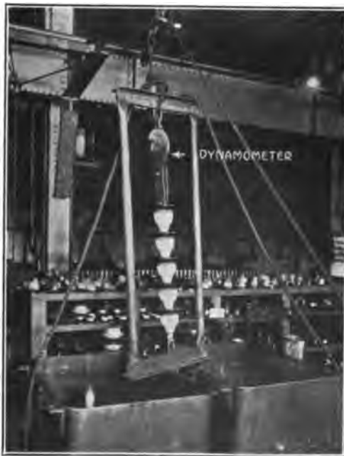
FIG. 17—TESTING INSULATORS BY TEMPERATURE CHANGES
