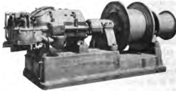
FIG. 2—NEW TYPE OF ELECTRIC CARGO WINCH HAVING THE REDUCTION GEAR INSIDE THE DRUM
