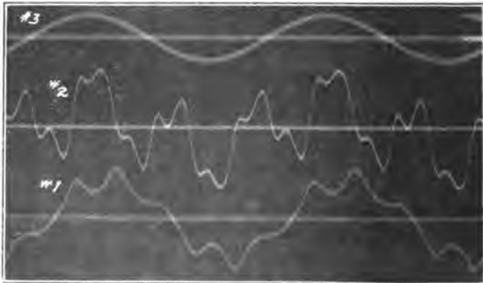
FIG. 12—Δ Y TRANSFORMERS AND LINES—NO STEP-DOWN TRANSFORMERS
