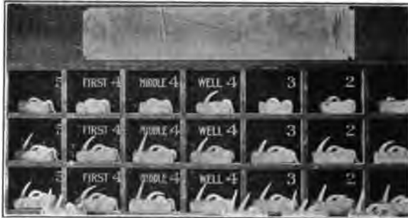
FIG. 12—TYPICAL PHOTOGRAPHIC RECORD OF KILN FIRING
