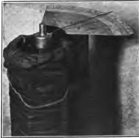
FIG. 2—SUSPENSION OF CABLE SAMPLE IN FIELD, SHOWING BIPILAR SUSPENSION AND SCALE FOR MEASURING DEFLECTIONS
