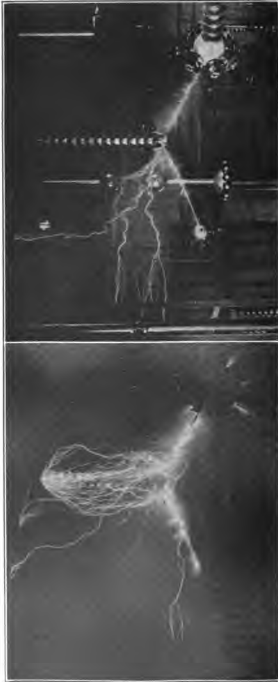
FIG. 20—TEST WITH 500,000-CIR. MIL. P. G. & E. CONDUCTOR. 14-UNIT STRING, NO. 25620
