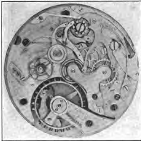
FIG. 15—SPLIT SECONDS SWISS WATCH WHICH HAS ONLY THE TWO SWEEP SECOND HANDS AND MINUTE HAND
