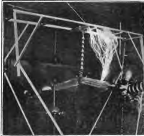
FIG. 6—SAME INSULATOR STRING. 514 Kv.—34,000 CYCLES. INSULATED CONTROLS AND CONDUCTOR GUARD
