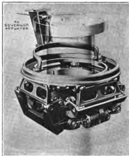
FIG. 12—DIRECT-CONNECTED FLYBALL GOVERNOR For mounting on the main shaft.
