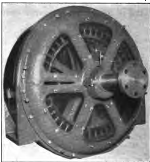
FIG. 4—COUPLING END OF 46-POLE, 2600-H. P., 50-CYCLE, 130-REV. PER MIN., SYNCHRONOUS MOTOR FOR SHIP PROPULSION
