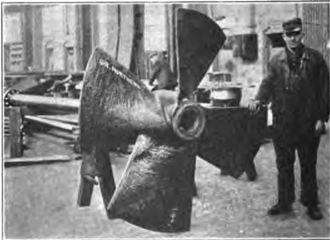
1 G. 6—SHOP VIEW OF 72-IN. HIGH-SPEED CAST STEEL RUNNER Assembled on shaft and showing initial stages of assembling for balancing before finally grinding to a surface. Designed for 600-h. p., 200-rev. per min., 17½-ft. head.
