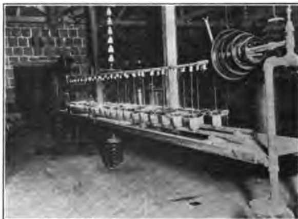
FIG. 14—ROUTINE ELECTRICAL TEST OF PORCELAIN PARTS
