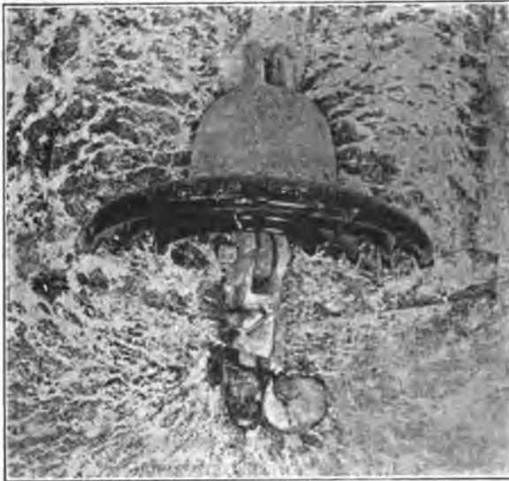
FIG. 15—DIELECTRIC FIELD OF CAP AND PIN SUSPENSION INSULATOR
