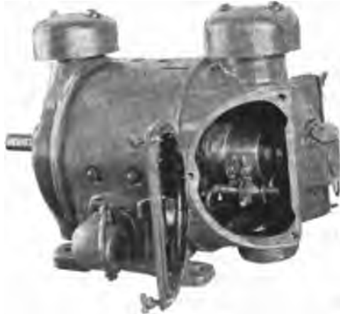
FIG. 5—MARINE D-C. MOTOR—ENCLOSED, VENTILATED, FOR OPERATING BELOW-DECK MACHINERY
