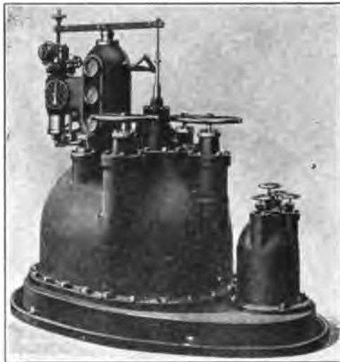
FIG. 13—SPECIAL CENTRIFUGAL CONTROL STAND FOR TYPE NO. 4 ALLIS-CHALMERS HYDRAULIC TURBINE OIL PRESSURE GOVERNOR USED IN CONNECTION WITH FLYBALLS MOUNTED ON THE TURBINE MAIN SHAFT BELOW THE GENERATOR
