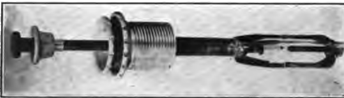
FIG. 10—MECHANISM FOR 200-AMPERE MEDIUM INTENSITY ARC, AS USED IN OPEN TYPE SEARCHLIGHT
