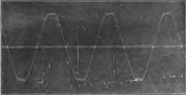
FIG. 2—OPEN CIRCUIT VOLTAGE—EXAMPLE 1 (EFFECTIVE VALUE, 100 VOLTS)
