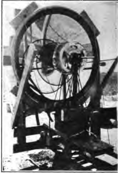
FIG. 7—ORIGINAL OPEN TYPE SEARCHLIGHT, WITH 36 IN. MIRROR AND 150-AMPERE HIGH INTENSITY ARC, AUTOMATICALLY OPERATED MECHANISM
