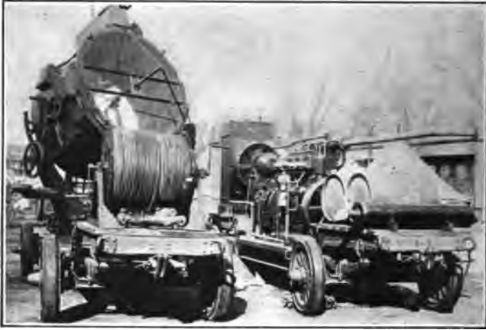
FIG. 3—TRAILER TYPE OF MOBILE SEARCHLIGHT EQUIPMENT, CONSISTING OF 60 IN. BARRELL SEARCHLIGHT AND 25-KW., 125-VOLT GASOLINE-ELECTRIC GENERATING SET.
