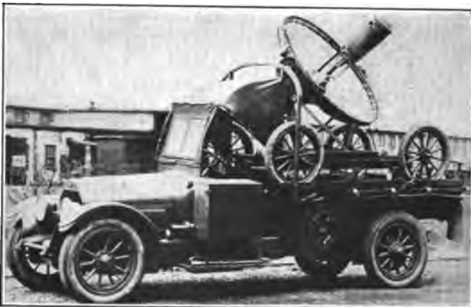
FIG. 16—LATE 1918 DESIGN OF MOBILE SEARCHLIGHT POWER UNIT AND LORRY, WITH COVERS REMOVED, SHOWING SEARCHLIGHT IN POSITION
