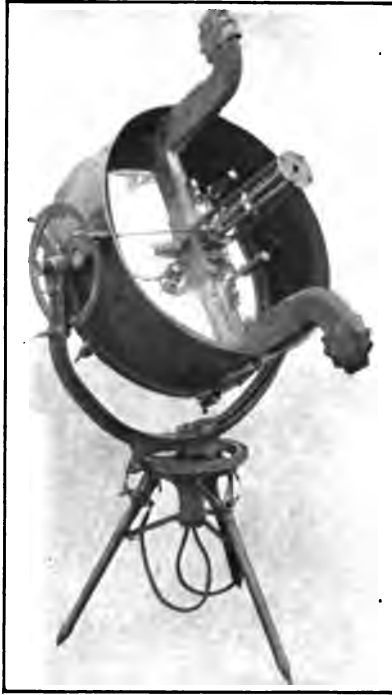
FIG. 12—VERY LIGHT WEIGHT MODEL OPEN TYPE SEARCHLIGHT, WITH 30 IN. MIRROR AND 150-AMPERE HIGH INTENSITY ARC, HAND FEED MECHANISM
