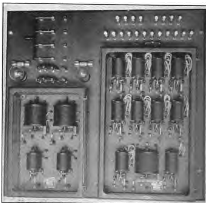
FIG. 9—COMBINED CURRENT AND VOLTAGE REGULATORS FOR 'HIGH-FREQUENCY ALTERNATOR CONTROL
