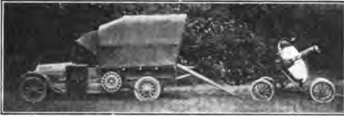
FIG. 14—LATE 1918 DESIGN MOBILE SEARCHLIGHT POWER UNIT AND LORRY, WITH 60 IN. OPEN TYPE SEARCHLIGHT
