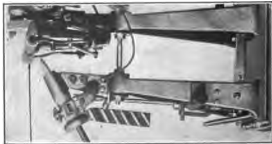
FIG. 7—SEARCHLIGHT LAMP WITH THIRD ELECTRODE CONTROL
