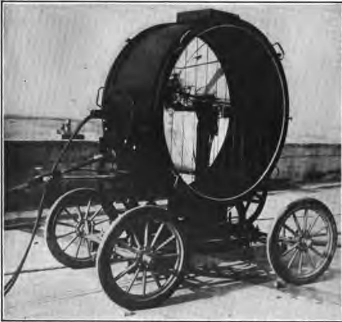
FIG. 6—60 IN. HIGH INTENSITY ARC, LIGHT WEIGHT, BARREL SEARCHLIGHT ON WHEELED BASE
