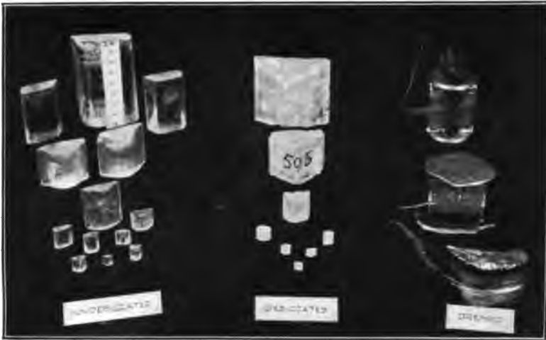
FIG. 6—GROUP OF ROCHELLE SALT CRYSTALS—UNDESICCATED, DESICCATED AND DRESSED
