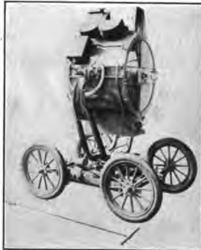
FIG. 2—36-IN. BARREL TYPE WHEELED BASE SEARCHLIGHT, SUCH AS USED BY 1ST AND 2ND FIELD ARMIES, A. E. F.
