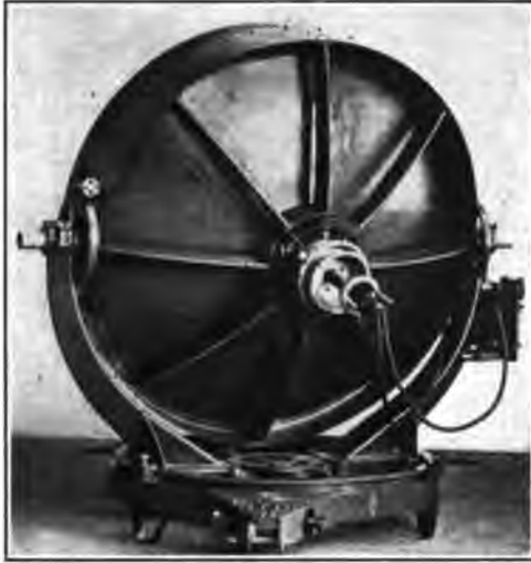
FIG. 9—1919 MODEL OF OPEN TYPE SEARCHLIGHT, WITH 60 IN. MIRROR, SHOWING WHEELS REMOVED AND BASE READY FOR EMPLACING
