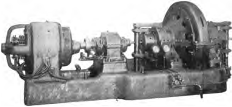
FIG. 4—50-Kw. 50,000-CYCLE ALTERNATOR
