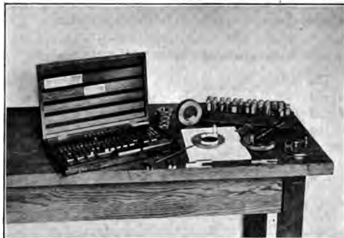
FIG. 9 THREE-BALL METHOD OF MEASURING THE EFFECTIVE DIAMETER OF A RING THREAD GAGE
