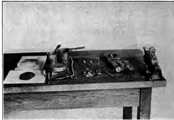
FIG. 8 CASTS OF THREAD AND APPARATUS USED IN MAKING THEM
