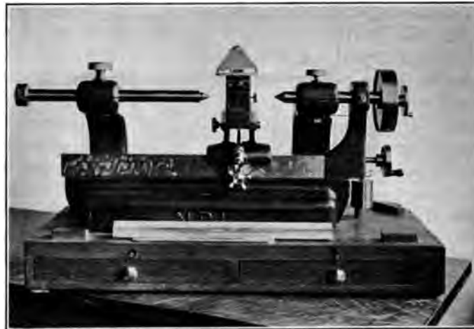
FIG. 2 PITCH-MEASURING MACHINE RECENTLY DEVELOPED BY THE NATIONAL PHYSICAL LABORATORY
