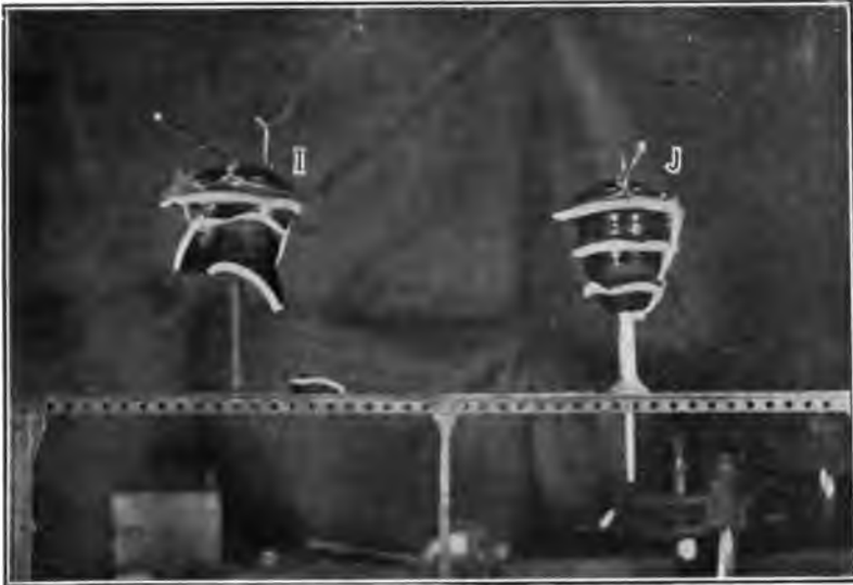
FIG. 32—ALL SHEDS BROKEN—60-CYCLE DRY FLASHOVER
