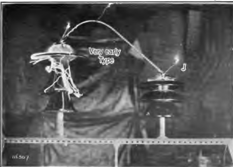
FIG. 25—60-CYCLE DRY FLASHOVER
