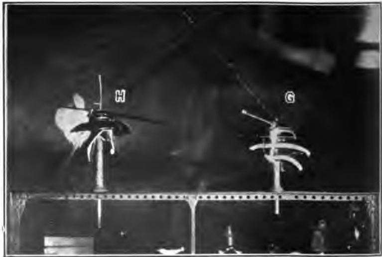
FIG. 31—SECOND AND THIRD SHEDS BROKEN—60-CYCLE DRY FLASHOVER
