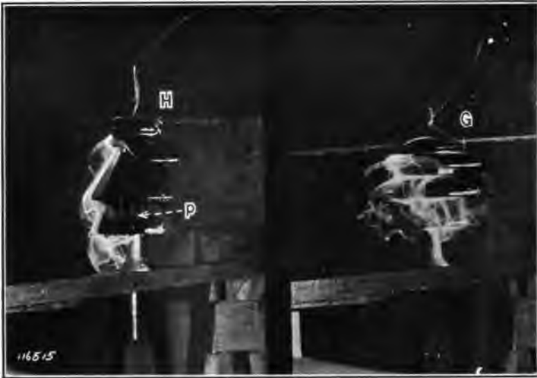
FIG. 28—TOP SHED BROKEN—60-CYCLE WET FLASHOVER
