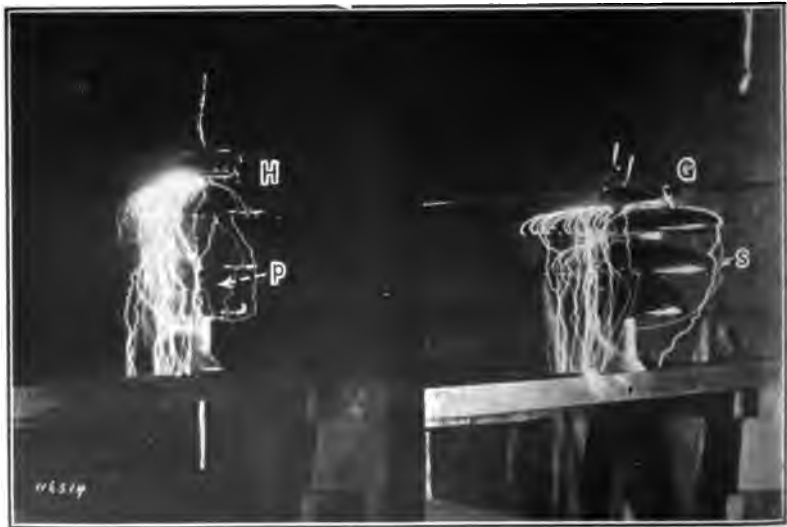
FIG. 23—60-CYCLE WET FLASHOVER
