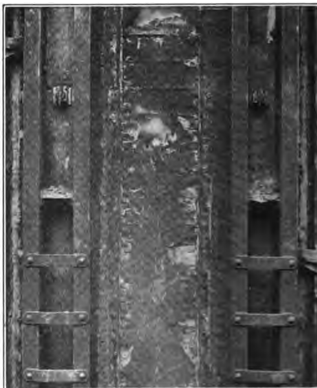
FIG. 4 COKE IN BY-PRODUCT OVEN JUST AFTER REMOVING DOOR
