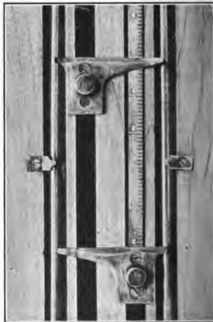
FIG. 6 ENLARGED VIEW OF SCALE AND POINTERS FOR U-TUBE IN FIG. 5
