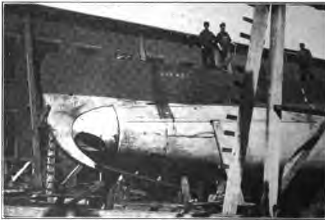
FIG. 5 BOW OF SUBMARINE WITH BOW CAP IN POSITION FOR TORPEDO FIRING
