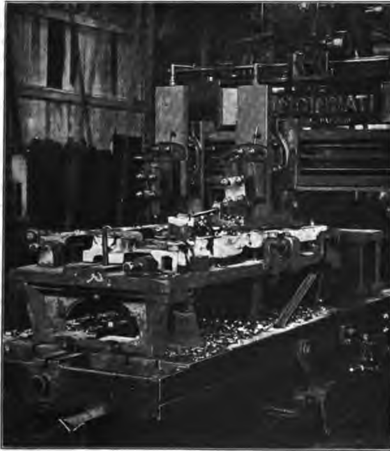
FIG. 1 EXAMPLE OF TIME-SAVING JIG ON PLANER
