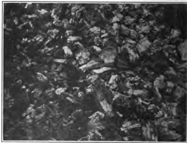
FIG. 25 COKE FROM SAME COAL AS FIG. 24, PROPERLY MADE
