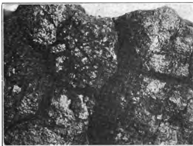
FIG. 7 WALL END OF A BLOCK OF COKE
