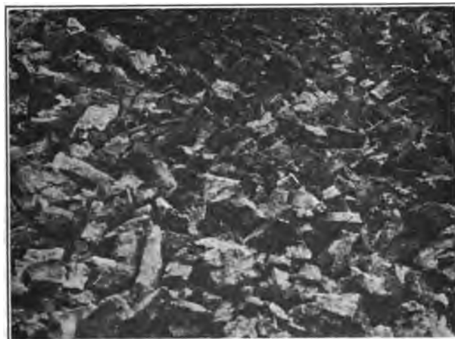
FIG. 23 COKE FROM SAME COAL AS FIG. 22, WITH 20 PER CENT POCAHONTAS
