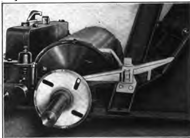
FIG. 3 INTERLOCKING DEVICE FOR BEATER COVER AND DOOR OVER DIET GRID (PAT.)
