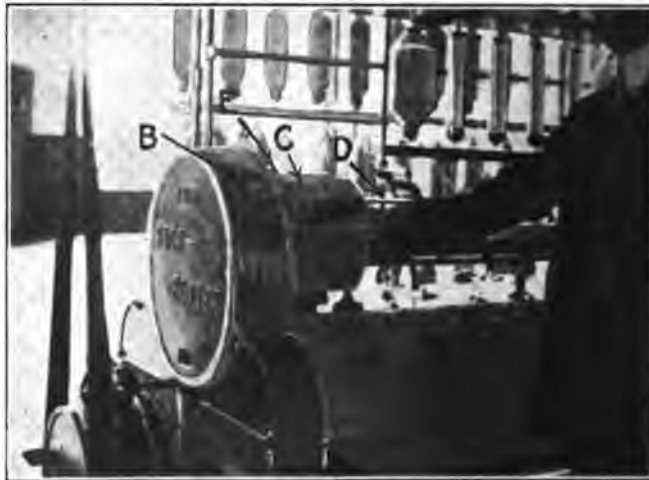
FIG. 9 INTERLOCKING GUARD FOR DRAFT GEARS OF ROVING FRAME
