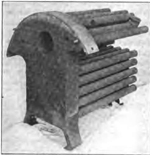
FIG. 8 SUPERHEATER REMOVED FROM BOILER
