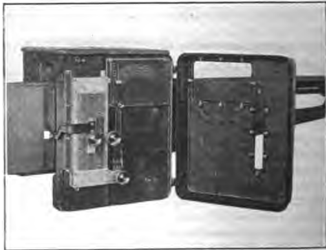
FIG. 17 PHOTOGRAPHIC VIEW OF VOLUME CORRECTOR Front door of casing opened
