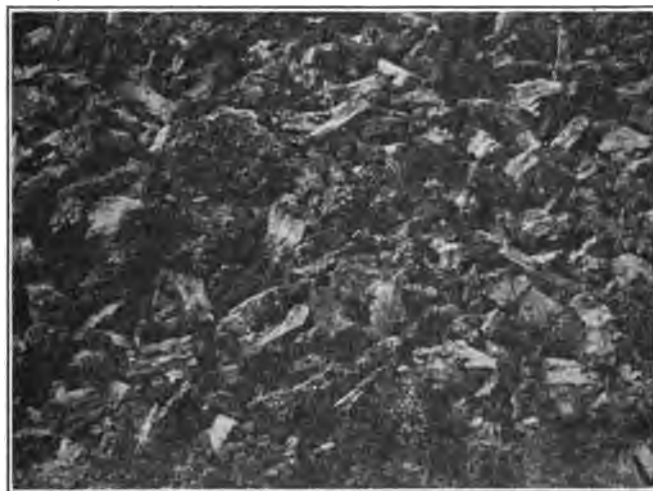
FIG. 22 COKE FROM STRAIGHT HIGH-VOLATILE COAL, SHOWING SPONGE
