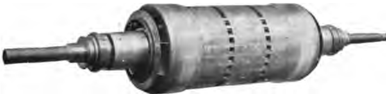
THE SAME TYPE FOR 600 KV-A.—3600-REV. PER MIN.—BUILT IN CINCINNATI IN 1904
