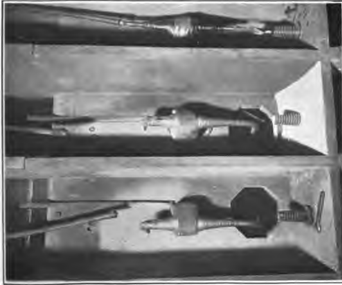
FIG. 2—BURNED OFF LINE LEADS
