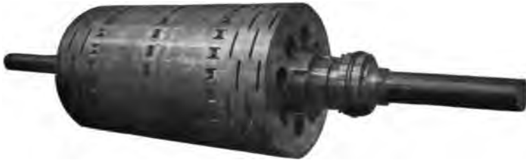
THE ORIGINAL 1500-KV-A.—1500-REV. PER MIN.—RADIAL-SLOT TURBO ROTOR, BUILT IN CINCINNATI IN 1902-1903—THE FIRST STEP IN THE EVOLUTION OF THE TYPE
