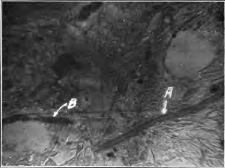
FIG. 8—300 DIAMETERS—TAKEN FROM A SUSPENSION UNIT REMOVED FROM THE LINE FOR LOW MEGGER READING AFTER ELEVEN MONTHS SERVICE
