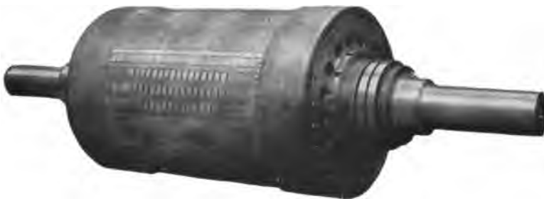
[BEHREND] RADIAL SLOT PLATE ROTOR WITH BOLTED FORGED SHAFT ENDS— 25,000 KV-A.—1500-REV. PER MIN.—BUILT IN PITTSBURGH IN 1916
