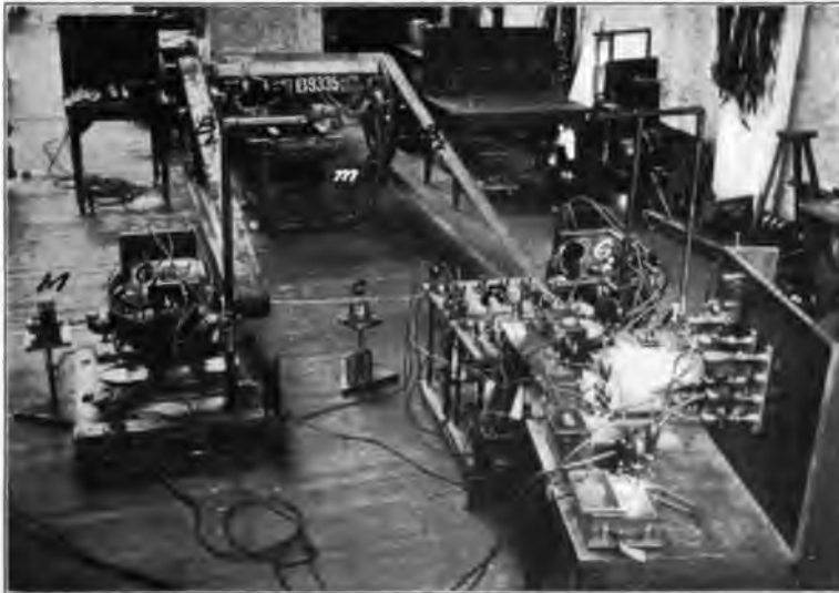
FIG. 8—VIEW OF TEST ARRANGEMENT FOR TRUCK EFFICIENCY
