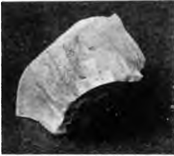
FIG. 2—FRACTURES FROM ZONE A-B INSULATOR NO. 1. TWO AND ONE-HALF DIAMETERS — INNER PETTICOAT
