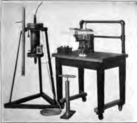
[WHITEHEAD] FIG. 3—CORONA VOLTMETER FOR 50,000 VOLTS
