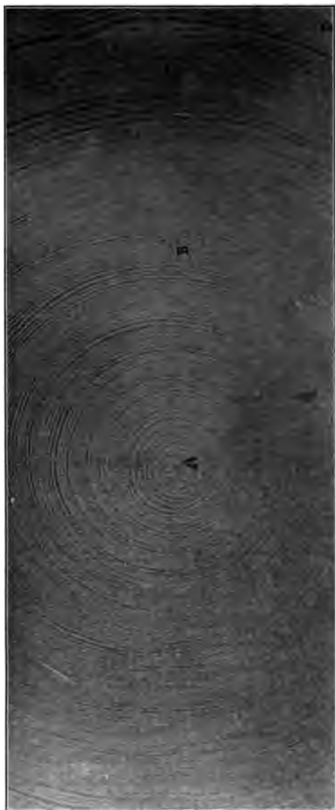
FIG. 1 LONGLEAF PINE, 8 IN. BY 18 IN. DISTRIBUTION OF RESIN: A 25 PER CENT, B 14 PER CENT, C 17 PER CENT, D (SAPWOOD) 3 PER CENT
