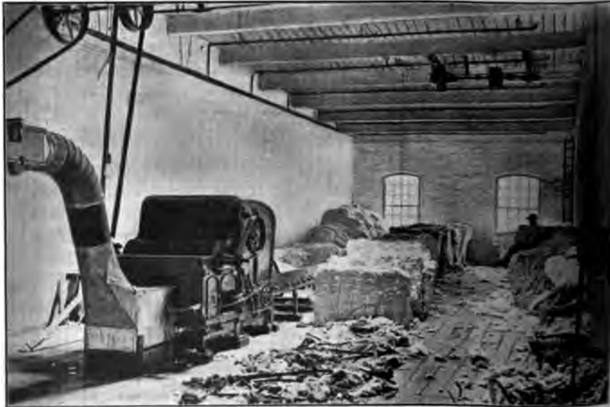
FIG. 2 OPENING ROOM WITH BALE BREAKER DELIVERING TO A CONVEYOR PIPE UNDER SUCTION, WITH BOX TO CATCH HEAVY MATERIAL
