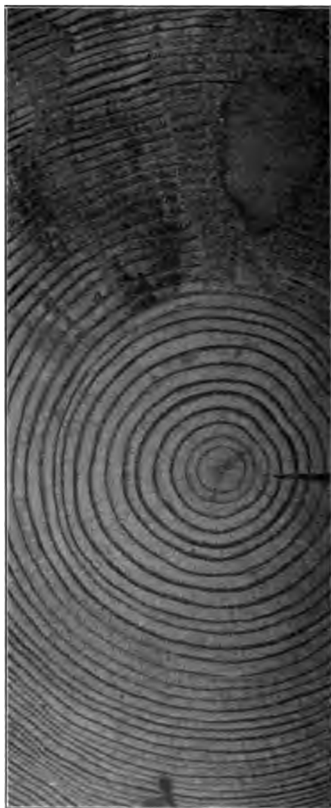
FIG. 3 NORTH CAROLINA, OR LOBLOLLY, PINE, 8 IN. BY 18 IN. WITH ROT IN NON-RESINOUS WOOD
