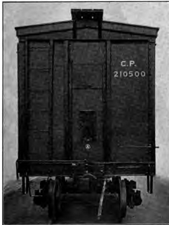
FIG. 4 END VIEW OF CANADIAN PACIFIC INSIDE SHEATHED CAR SHOWING GRAIN-TIGHT END DOORS
