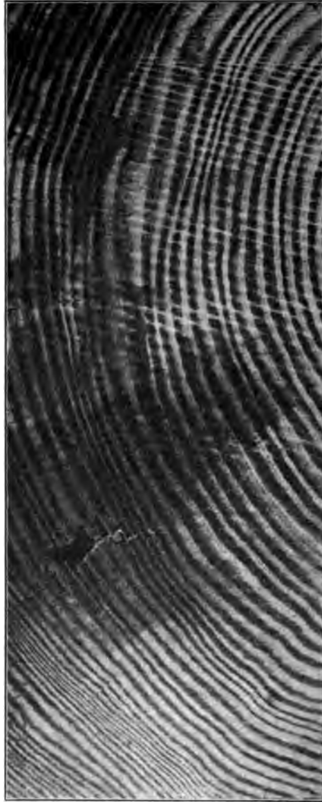
FIG. 2 CUBAN PINE, 8 IN. BY 18 IN. WITH ROT IN SAPWOOD
