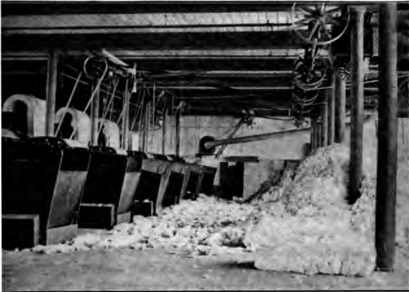
FIG. 3 PICKER ROOM WITH HOPPERS OF AUTOMATIC FEEDERS FILLED BY HAND FROM PILES FED FROM CONDENSERS ABOVE
