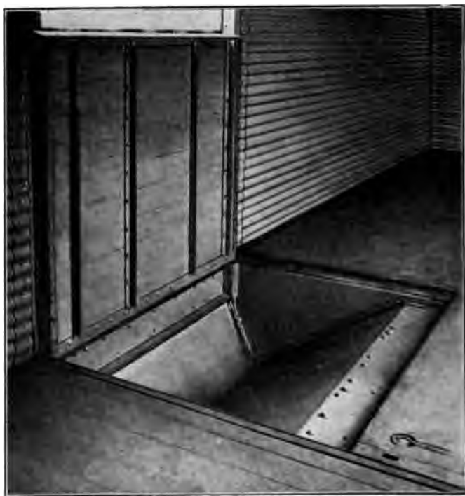
FIG. 10 DETAIL VIEW OF HOPPER OPENING IN FLOOR OF CORRUGATED STEEL LINED CAR
