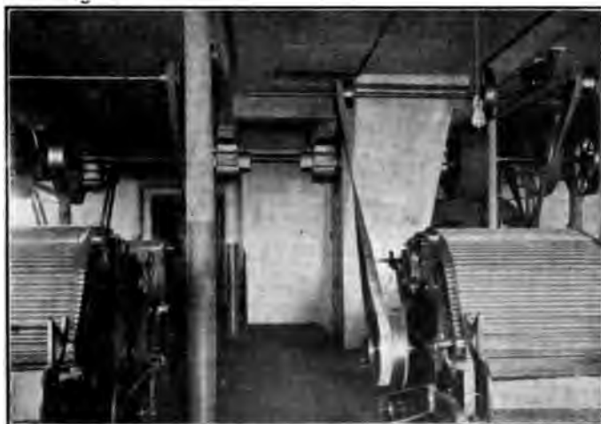
FIG. 8 CARD ROOM, THIRD STORY. END VIEW OF BELT ENCLOSURE. BEARINGS ALL OUTSIDE
