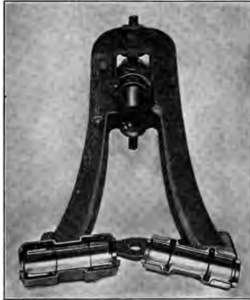
FIG. 4 TYPE OF RING-OILED BABBITT BEARING USED IN TESTS
