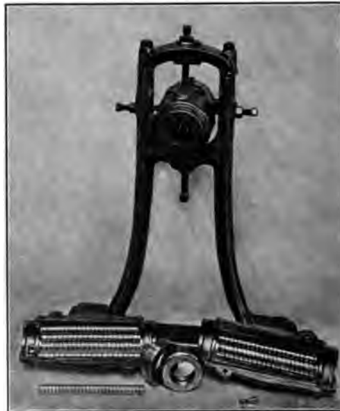
FIG. 5 TYPE OF ROLLER BEARING USED IN TESTS
