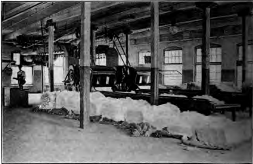
FIG. 1 OPENING ROOM HANDLING LARGE QUANTITIES OF COTTON FED BY HAND FROM THE BALES TO THE APRONS
