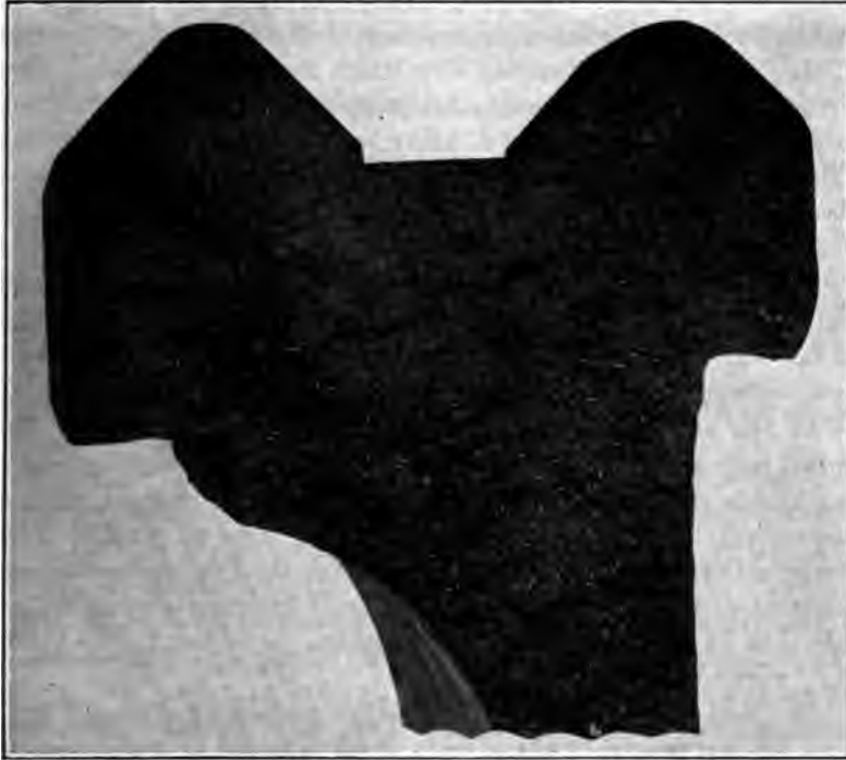
FIG. 2 CROSS-SECTIONAL FRACTURE OF CHILLED LATHE-BED
