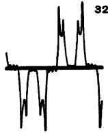
CURVE 32.—POTENTIAL WAVE ON EXPLORING COIL, SPANNING 1 TOOTH OF 12 SLOTS PER POLE 1400 kv-a., 50 cycles, three-phase, 10,000 volts.
