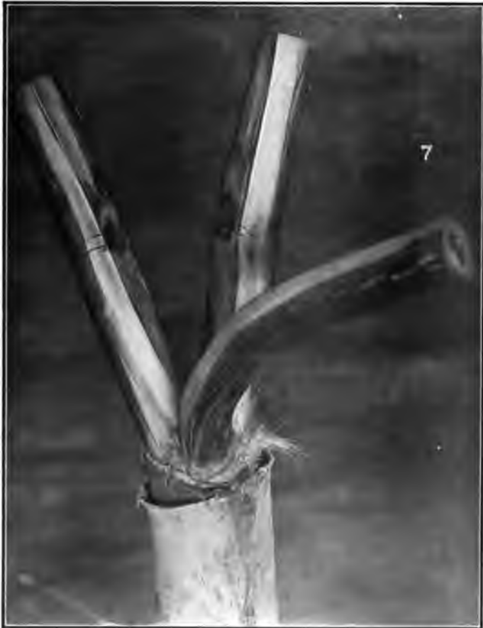
FIG. 7—CONDUCTORS SPREAD TO SHOW FAULT
