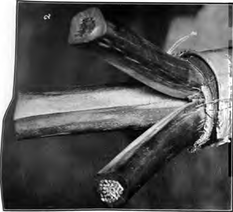
FIG. 2—18,000 VOLTS FOR 40 MINUTES [TORCHIO]
