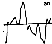
CURVE 30.—CURRENT WAVE BETWEEN SHAFT AND BEARING. 9375 kv-a., 60 cycle, three-phase, 5000 volts.
