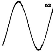
CURVE 52.—POTENTIAL WAVE — 100 PER CENT LOAD. 9 kv-a., 60 cycle, three-phase, induction motor, as generator, with d-c. excitation from all three phases of secondary.
