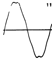
CURVE 11.—POTENTIAL WAVE—NO LOAD —DELTA CONNECTED 900 kv-a., 25 cycles, 150 rev. per. min., three- phase, 400 volts.
