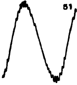
CURVE 51.—POTENTIAL WAVE—NO LOAD. 9 kv-a., 60 cycle, three phase, induction motor, as generator, with d-c. excitation from all three phases of secondary.
