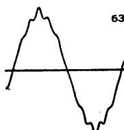
CURVE 63.—POTENTIAL WAVE — NO LOAD. 600 kv-a., 60 cycle, 600 rev. per. min., three-phase, 11,000 volts.
