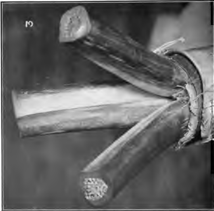
FIG. 3—18,000 VOLTS FOR 50 MINUTES [TORCHIO]
