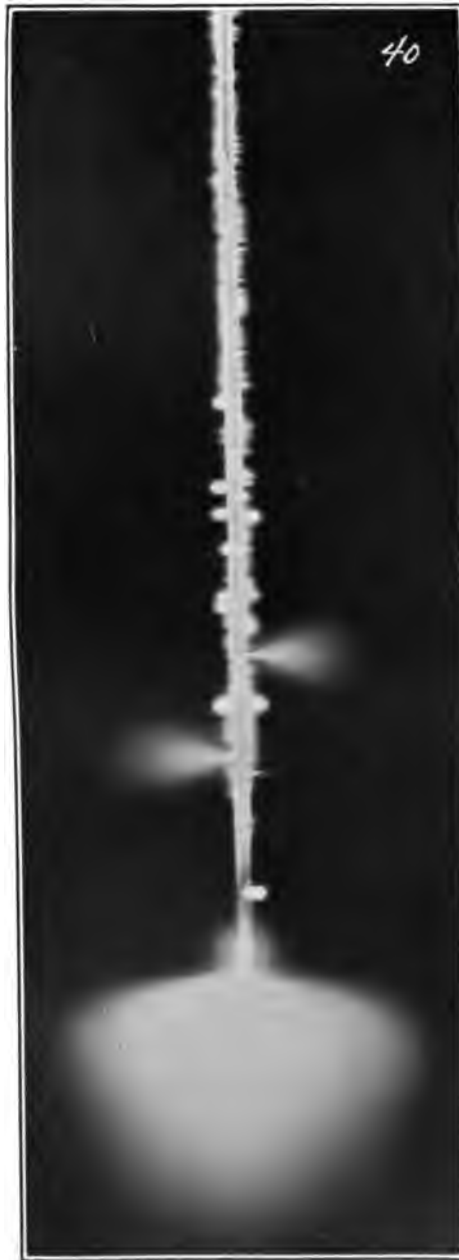
[PEEK] FIG. 40—ONE OF TWO PARALLEL STEEL RODS POINTED AT ENDS (DIRTY). Without stroboscope.
