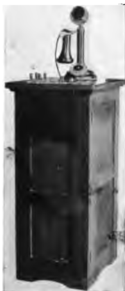
[DEAKIN] FIG. 4—COMMERCIAL EXCHANGE RECEIVING CABINET
