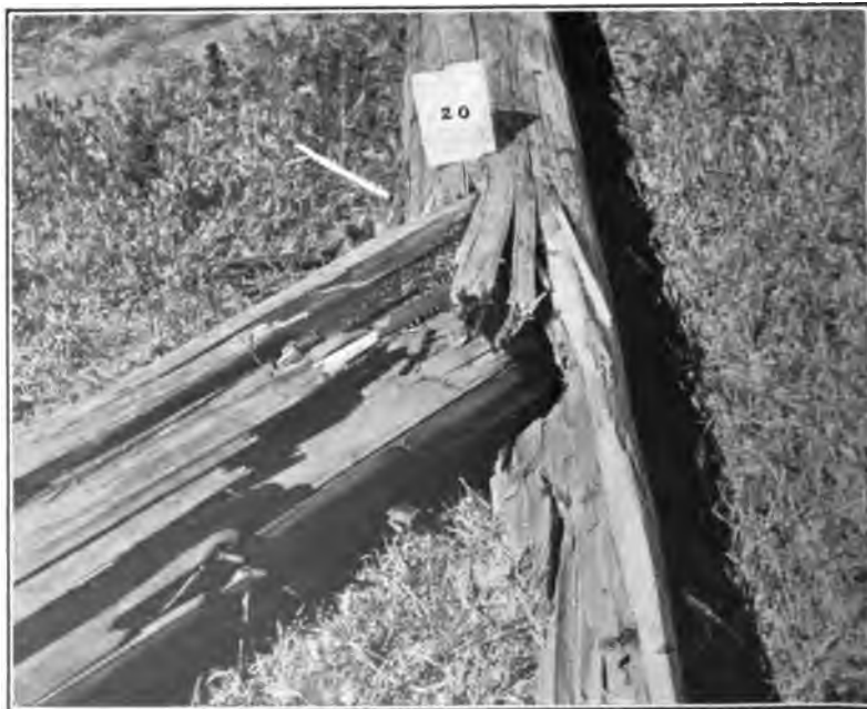
FIG. 10—SHOWING EFFECT OF EXCESS OF SAPWOOD, DUE TO RAPID GROWTH
