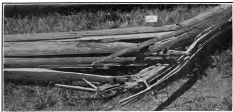
FIG. 7—TYPICAL BREAK OF PORT ORFORD CEDAR
