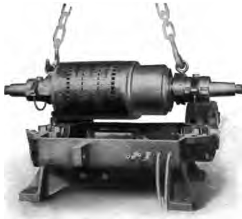
FIG. 2—REMOVING ARMATURE AND BEARINGS [WILEY]
