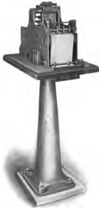
[CREIGHTON, NICHOLS AND HOSEGOOD] FIG. 9—FRONT VIEW OF THE PENCIL TYPE MULTI-RECORDER.
