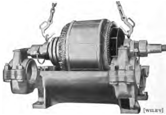
[WILEY] FIG. 10—LIFTING ROTOR AND STATOR FROM FRAME, A-C. MILL TYPE MOTOR
