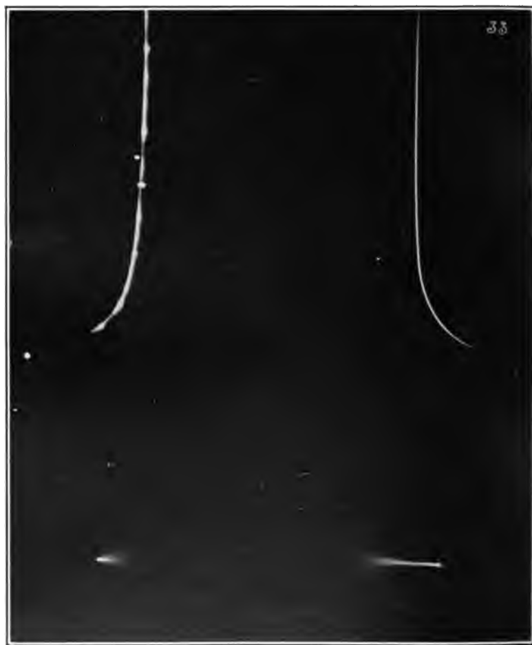
FIG. 33—COMPARISON OF CORONA ON WIRES AND BETWEEN NEEDLES, WITH STROBOSCOPE.
