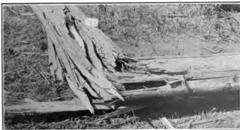
FIG. 8—TYPICAL BREAK OF WESTERN CEDAR FROM WASHINGTON
