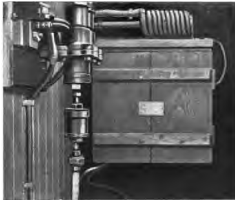
FIG. 9—DIRECT-CURRENT ALUMINUM ARRESTER AND CHOKE COIL INSTALLED IN MOTORMAN'S VESTIBULE.
