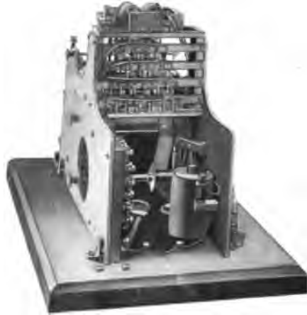
[CREIGHTON, NICHOLS AND HOSEGOOD] FIG. 8—BACK VIEW OF THE PENCIL TYPE OF MULTI-RECORDER.
