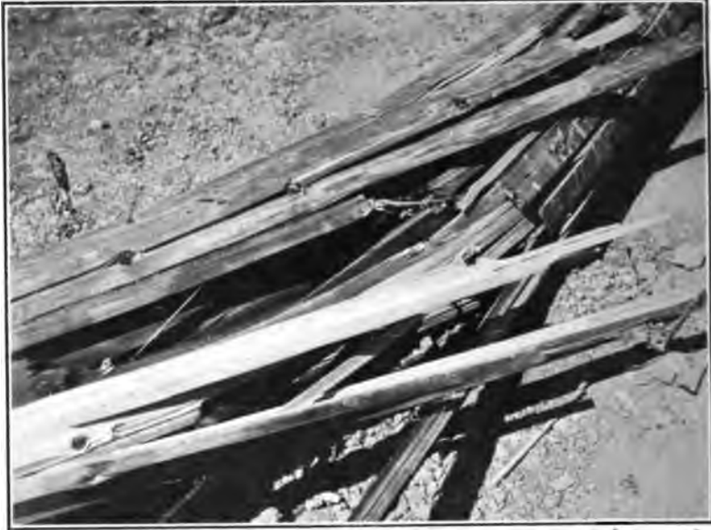
FIG. 9—EFFECT OF AXE-CUTS IN LOCATING POINT OF FRACTURE
