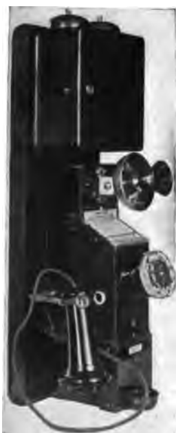
[DEAKIN] FIG. 1—PUBLIC TELEPHONE Equipped with 3-slot prepayment coin machine
