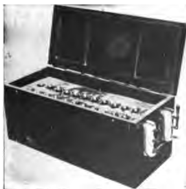
[DEAKIN] FIG. 9—PORTABLE STORAGE BATTERY
