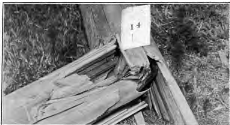
FIG. 6—TYPICAL BREAK OF WESTERN CEDAR FROM IDAHO
