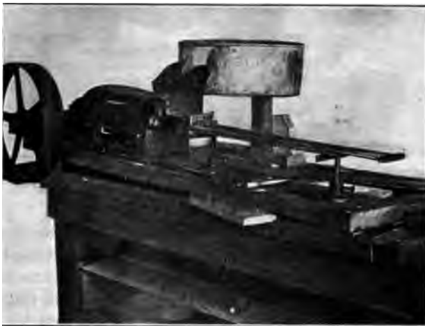
PLUNGER CORE MACHINE FITTED FOR MAKING 1-IN. SQ. CORES
