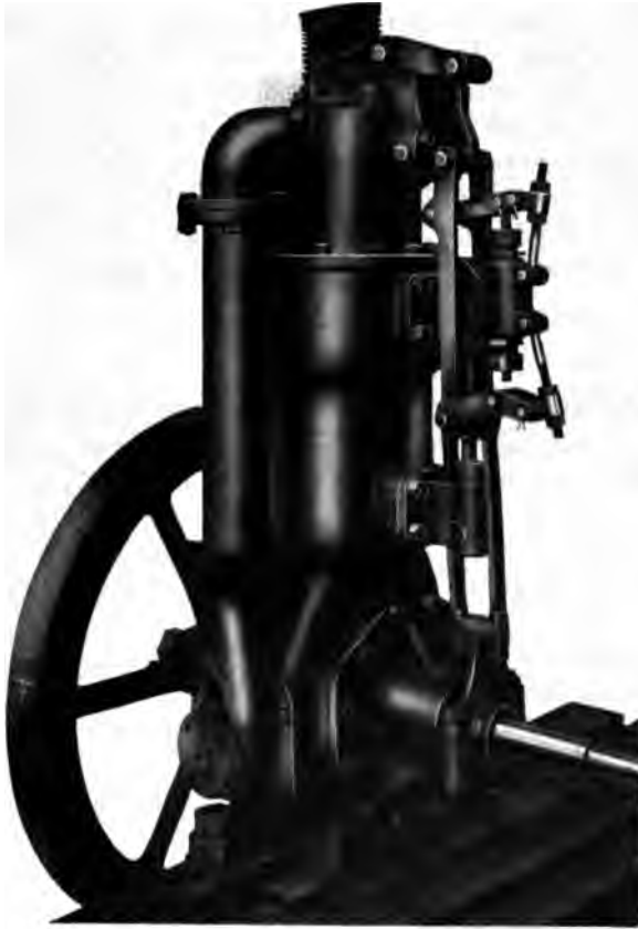
FIG. 28 SETZ ENGINE STANDING ON TESTING BLOCK
