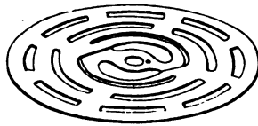
FIG. 19 MULTI-PORTED PLATE VALVE (HOERBIGER-ROGLER)
