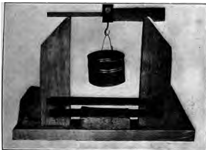
FIG. 8 DEVICE FOR BREAKING 1-IN. SQ. CORES
