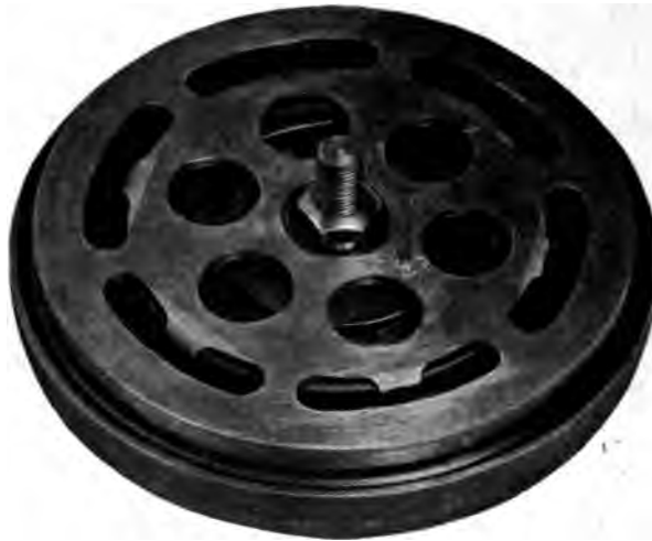
FIG. 25 MULTI-PORTED PLATE VALVES (MESTA)
