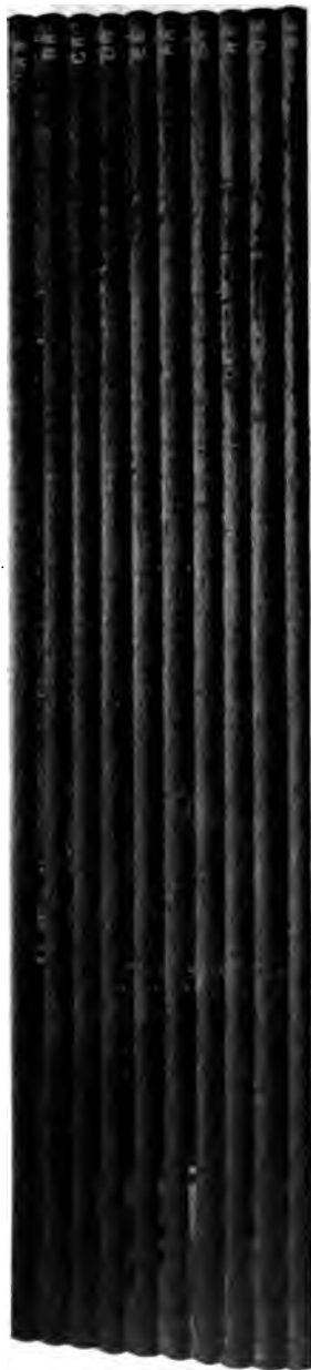
FIG. 11 APPEARANCE OF TUBES, BOILER No. 4084, AFTER DISMANTLING. VERTICAL ROW, EIGHTH FROM RIGHT SIDE OF BOILER
