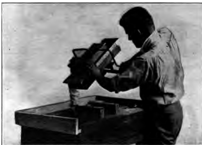
FIG. 5 DETROIT JAR-RAMMING CORE MACHINE IN THE ACT OF ROLLING OVER
