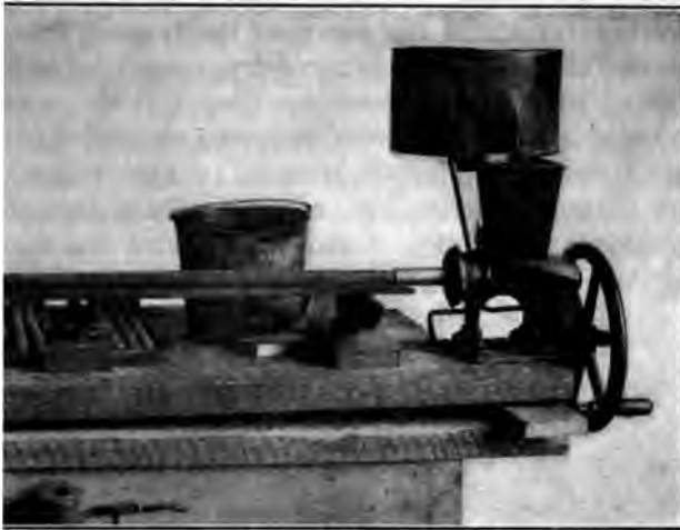
DSWORTH SCREW-FEED CORE MACHINE MAKING 1-IN. ROUND CORES
