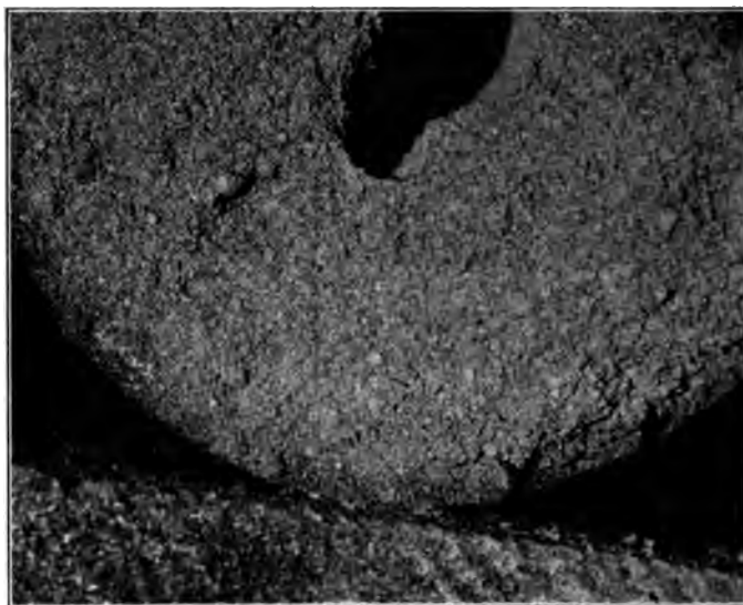
FIG. 17 CORE MADE FROM GANGWAY SAND WITH GLUTRIN AS A BINDER, SHOWING THE SWEATING OF THE BINDER TO THE SURFACE
