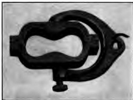
BOX OR MOLD USED FOR MAKING TEST CORES FOR TENSION TEST
