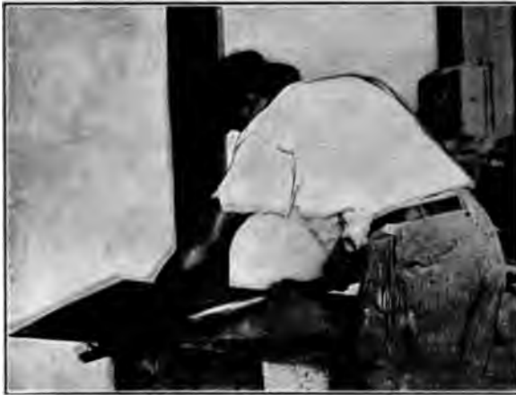
FIG. 1 MIXING SAND ON A PLATE WITH AN IRON PIPE
