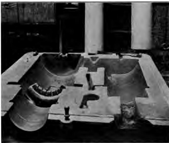
MOLD FOR LARGE 2-CYCLE GAS-ENGINE CYLINDER WITH PORT CORES IN PLACE, SHOWING SUPPORTERS FOR CORE ARBORS
