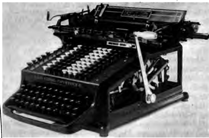
FIG. 7 THE ELLIS ADDING-TYPEWRITER WITH GLASS SIDES REMOVED
