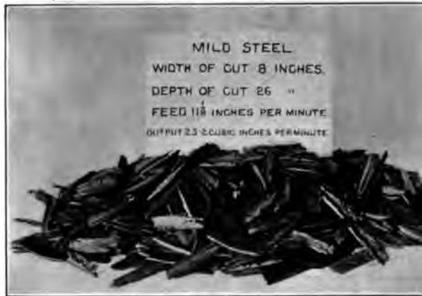
FIG. 48 EXAMPLE OF HEAVY MILLING PERFORMED BY NO. 3 PULLEY PLAIN MILLING MACHINE
