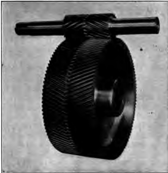
2 GEAR AND PINION FOR 200-H.P. TURBINE, TO RUN AT 5000 FT. PER MIN.
