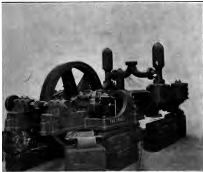
FIG. 13 GEAR-DRIVEN HORIZONTAL PUMP, GEAR RATIO 12\frac{1}{2} TO 1
