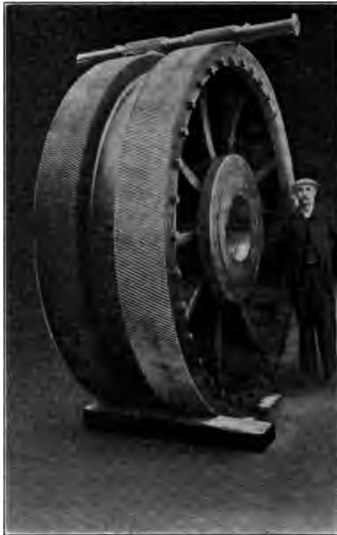
FIG. 8 GEAR AND PINION FOR 500-H.P. MARINE TURBINE
