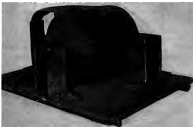
FIG. 39 PASTING JIG SHOWING COMPLETED CORE IN PLACE
