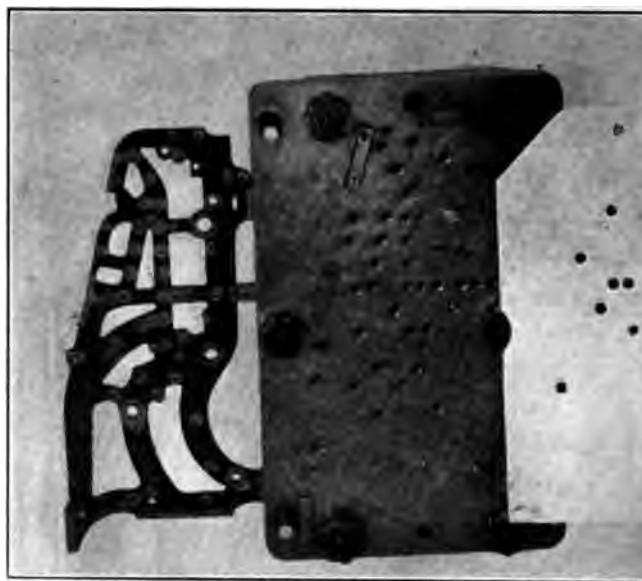
FIG. 13 LEFT SIDE FRAME B 47, DRILL JIG AND MASK
