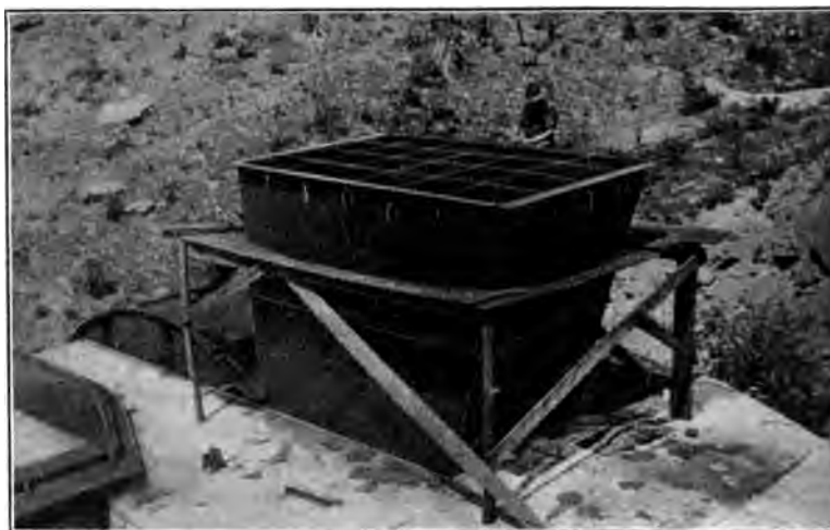
FIG. 12 DIVISION OF TOP OF CHIMNEY INTO EQUAL AREAS
