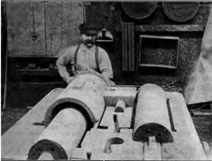
FIG. 43 MOLD FOR 2-CYCLE GAS-ENGINE CYLINDER, CORES SET
