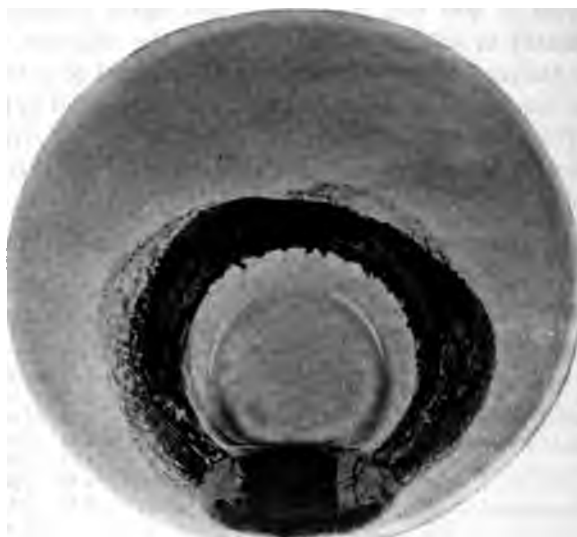
FIG. 18 RAW LINSEED OIL TESTED FOR DRYING QUALITIES
