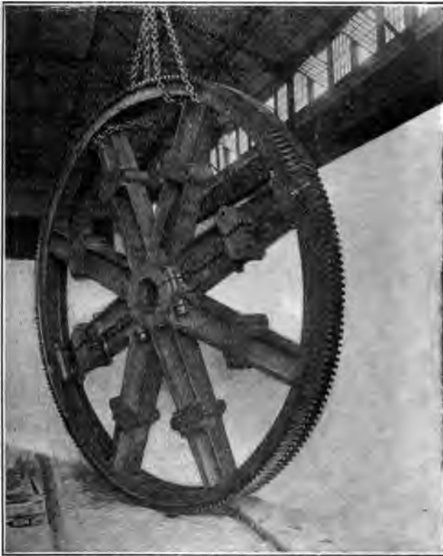
15 SEMI-STEEL GEAR, 12-IN. FACE, 12 FT. IN DIAMETER, FOR MINE HOIST
