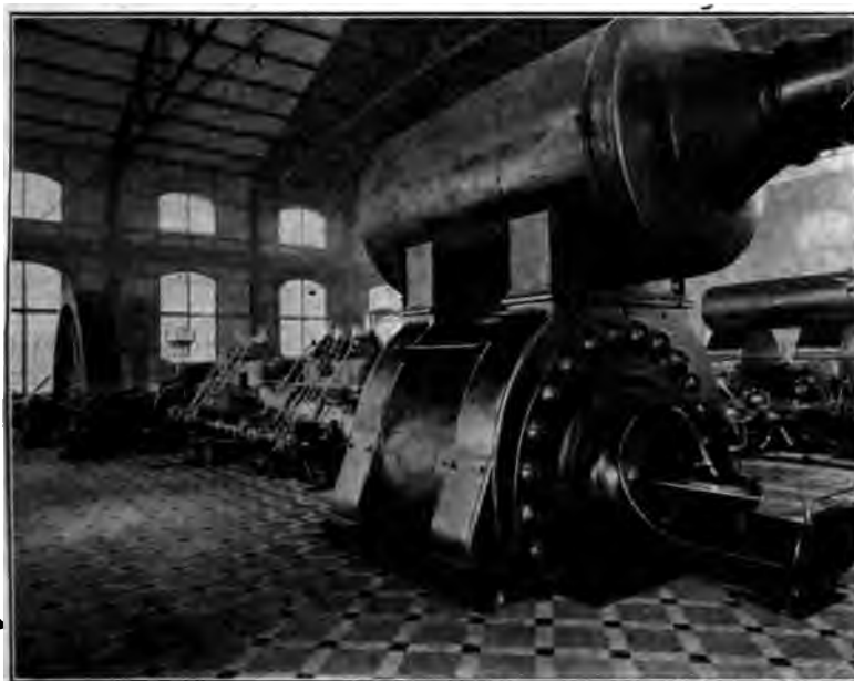
FIG. 29 BLOWING ENGINE WITH AIR TANK ON CYLINDER
