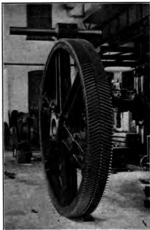
FIG. 17 HIGH RATIO PUMP GEARS, GEAR 9 FT. IN DIAMETER
