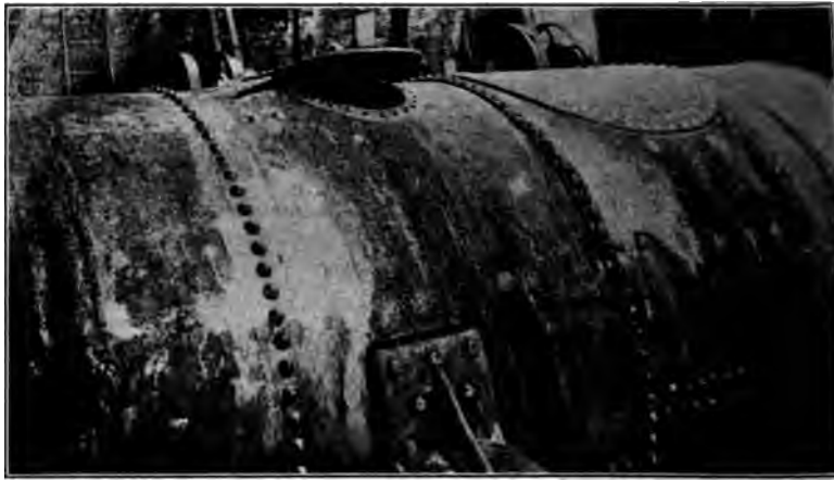
FIG. 28 MANHOLE PATCH AFTER RUPTURE. MAXIMUM-PRESSURE ON SHELL 335 LB. PER SQ. IN.
