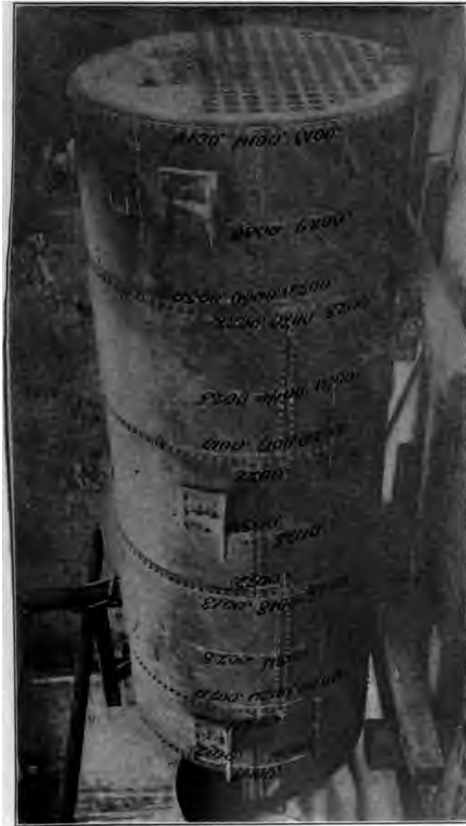
Fig. 33 TANGENTIAL EXTENSION AT 90 LB. PRESSURE. THE FIGURES GIVEN REPRESENT STRAINS DEVELOPED ON THE LEFT SIDE OF THE BOILER. NORMAL, COMPUTED EXTENSION AT THIS PRESSURE, 0.0029 IN.
