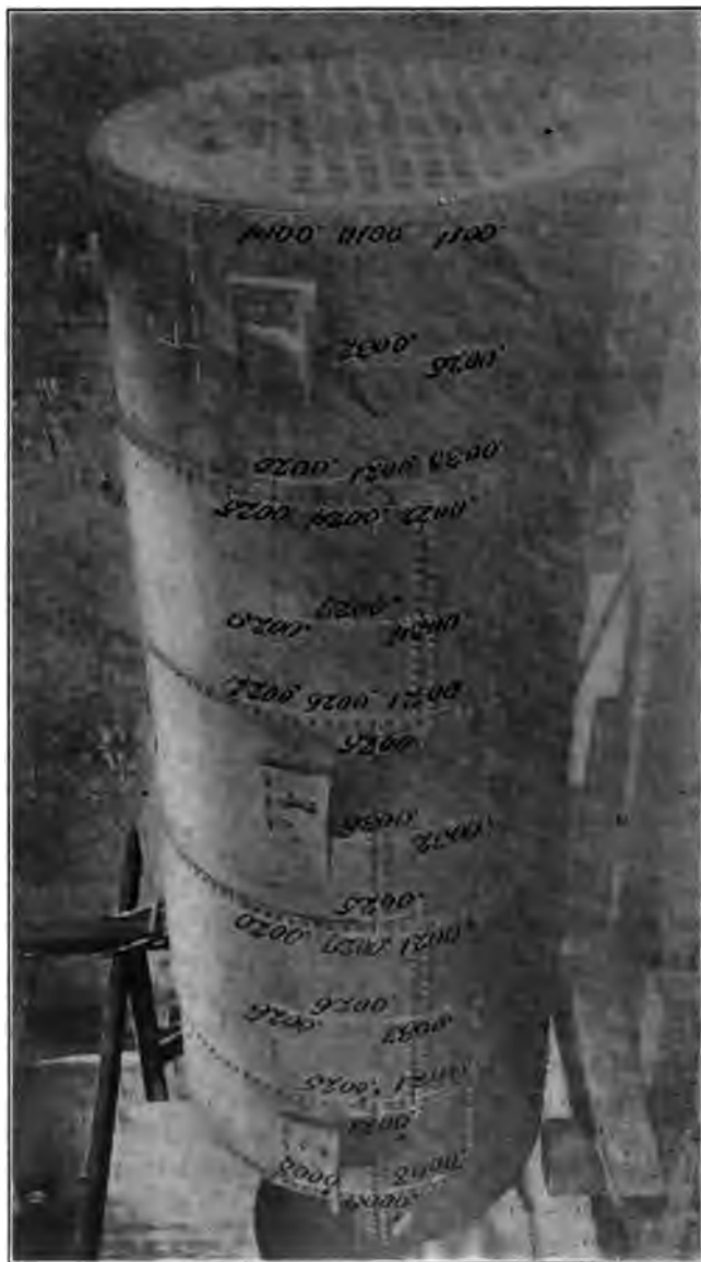
FIG. 32 TANGENTIAL EXTENSION AT 90 LB. PRESSURE. RIGHT SIDE OF BOILER. NORMAL, COMPUTED EXTENSION AT THIS PRESSURE, 0.0029 IN.
