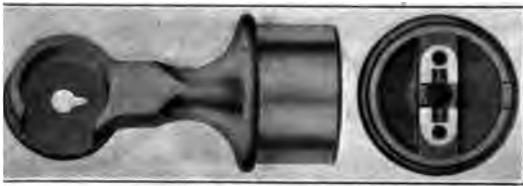
FIG. 6 HEAD FOR DESK TELEPHONE
