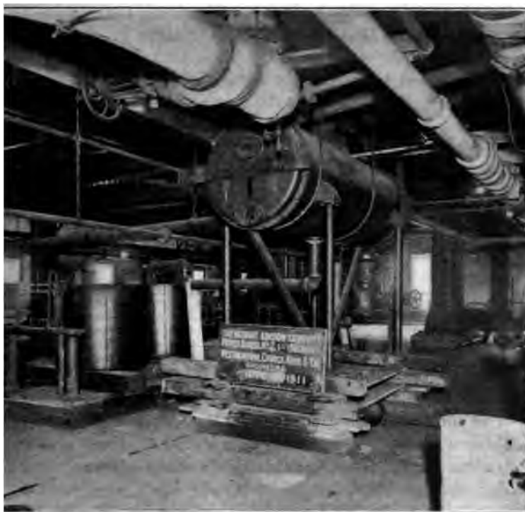
1) SPECIAL CONDENSER AND WEIGHING APPARATUS FOR DETERMINING QUANTITY OF STEAM USED BY STOKER AUXILIARIES .
