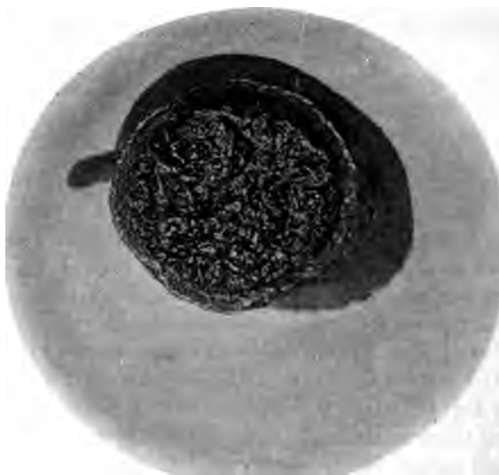
FIG. 19 CHINA WOOD OIL TESTED FOR DRYING QUALITIES
