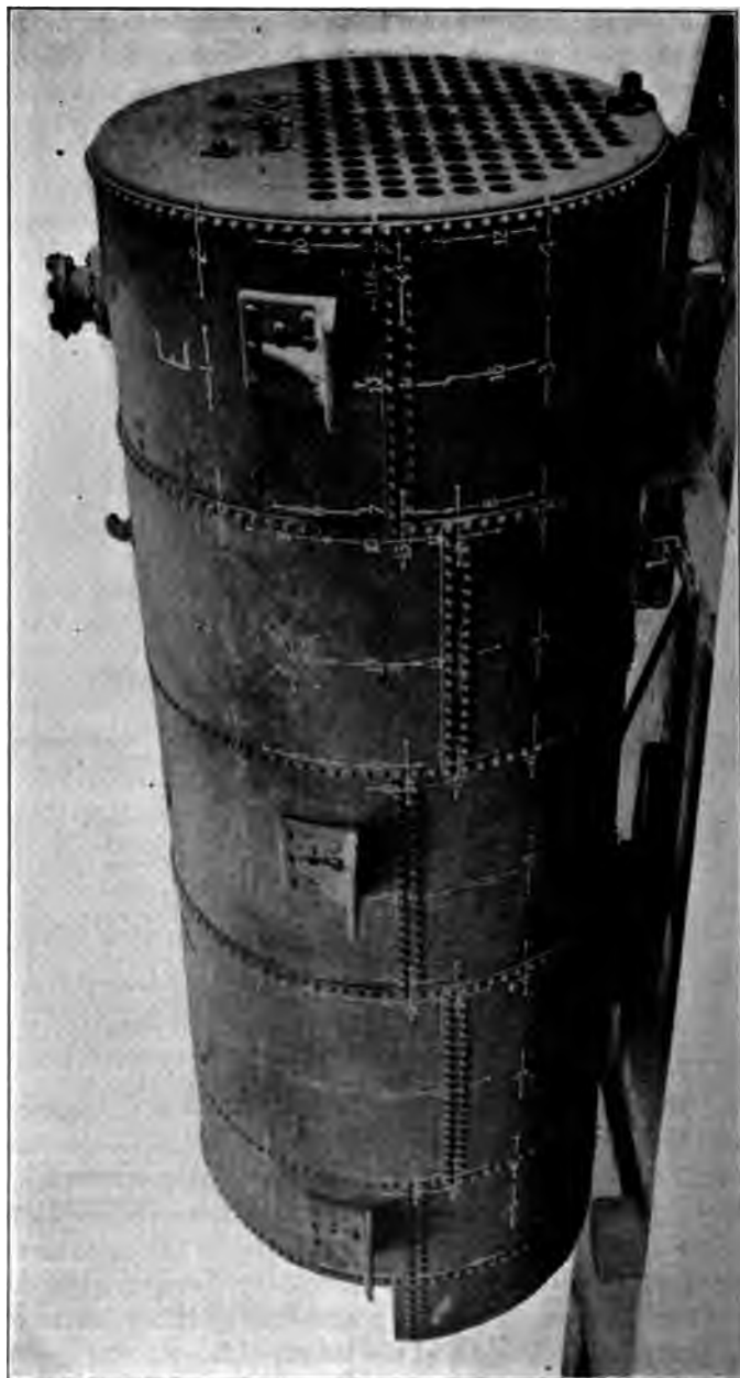
FIG. 14 STEAM BOILER, NO. 4002, DOME AND MANHOLE FRAME REMOVED PREPARATORY TO TESTING. HEADS STRENGTHENED WITH 6 THROUGH BRACES
