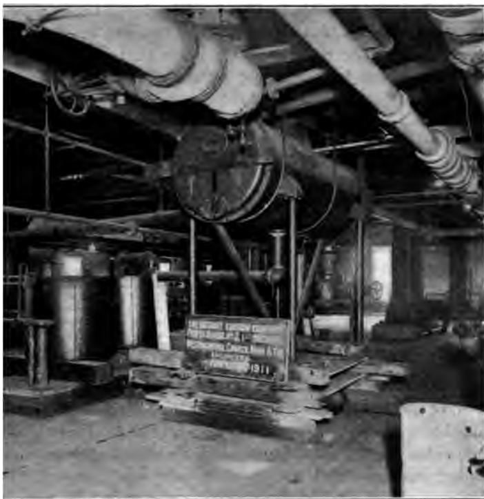
SPECIAL CONDENSER AND WEIGHING APPARATUS FOR DETERMINING QUANTITY OF STEAM USED BY STOKER AUXILIARIES
