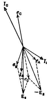
FIG. 14.—Two transformers cross-connected. Equal primary currents, 120 deg. apart. Secondary loads equal and of the same power factor
