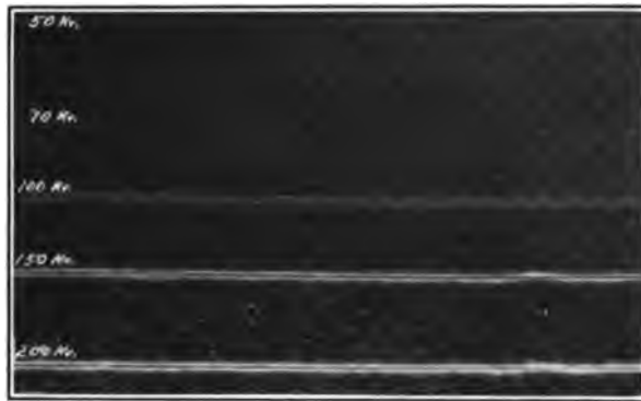
FIG. 44.—Polished copper wire. Diameter 0.186 cm. Polished after each exposure
