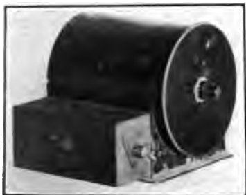
FIG. 13A.—Film holder with attachment for long films
