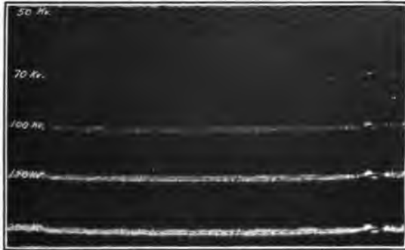
FIG. 46.—Weathered galvanized iron wire. Diameter 0.168 cm.
