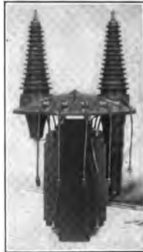
FIG. 7.—100-kw., 200,000-volt testing transformer—interior end view.
