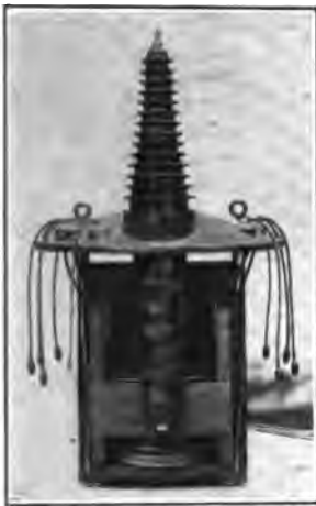
FIG. 6.—100-kw., 200,000-volt testing transformer—interior side view—showing voltmeter coil at center of high tension winding
