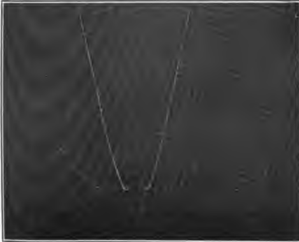
FIG. 2.—Corona on transmission line—No. 3/0 cable, 10-ft. spacing, 200,000 volts
