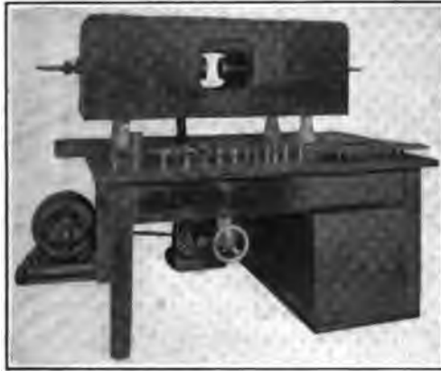
FIG. 15.—Spark gap for all high tension tests—showing different forms of electrodes employed and motor driven oil pump
