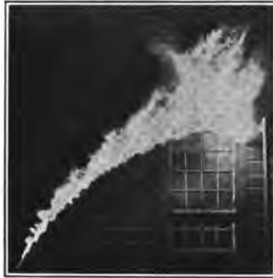
FIG. 3—Arc drawn by air-break disconnecting switch
