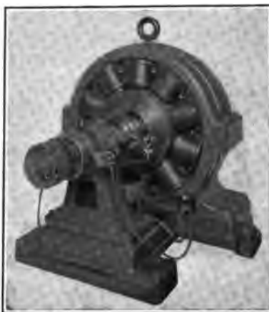
FIG. 3.—Thomson-Houston smooth core alternator—35 kw.—single-phase—125 cycles
