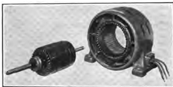
FIG. 1.—Sine-wave generator—distributed field type. 37.5 kw—three-phase—25 cycles
