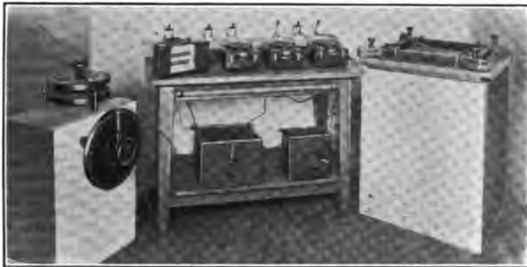
FIG. 4.—Apparatus for testing sheet iron
