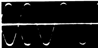
CURVE No. 129 Potential, line to line, 460 volts.
