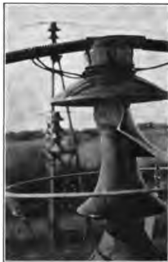
FIG. 16.—Insulator with second shell injured by lightning shock
