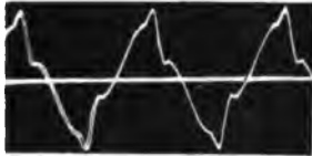
CURVE No. 99 Potential across one leg, 460 volts.
