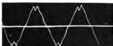
CURVE No. 171 Potential wave, neutral to line (no load), 2540 volts.
