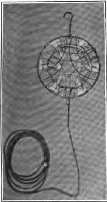
Lamp cluster used in tunnels and designed to reduce lamp breakage from blasting, etc., to a minimum.
