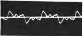
CURVE No. 91 Current in connected neutral, 3.5 amperes .
