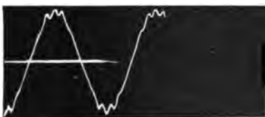
CURVE No. 173 Potential wave, neutral to line (no load), 2277 volts.
