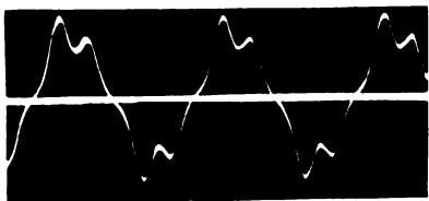
CURVE No. 127 Current in line 3, 9.7 am- peres.
