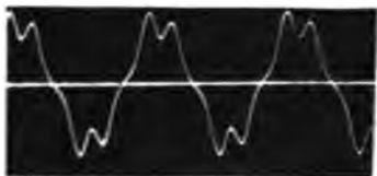
CURVE No. 130 Current in line 1, 11.4 amperes.
