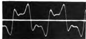
CURVE No. 97 Current in connected neutral, 24.9 amperes.
