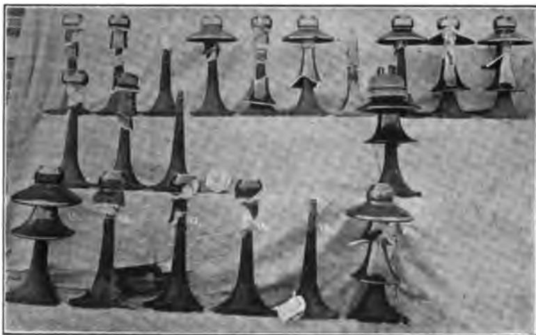
FIG. 6.—Insulators removed from the line after damage by lightning and power effects
