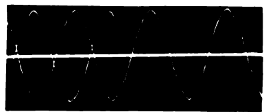
CURVE No. 166 Potential wave, neutral to line C (no load), 2455 volts.
