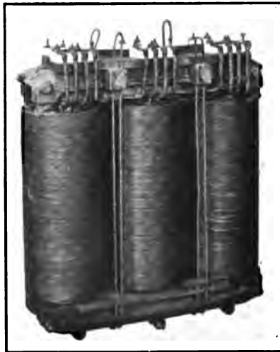
FIG. 26.—Three-phase, core-type, 25-cycle, 40-kw., 2300-volt primary, 460-volt secondary transformer used to investigate third harmonics
