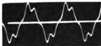
CURVE No. 132 Current in line 3, 9.7 amperes.
