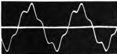
CURVE No. 107 Current in line 1, 2.0 am- peres.
