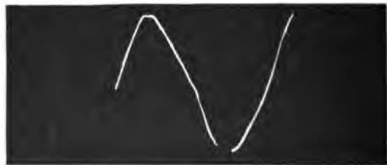
CURVE No. 177 Potential wave, ground to line (load, 500 kw.), synchronous mo- tor and 450-kw. transformer, 2473 volts.
