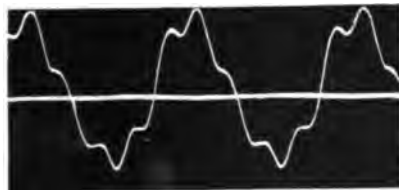
CURVE No. 108 Current in line 2, 1.92 am- peres.
