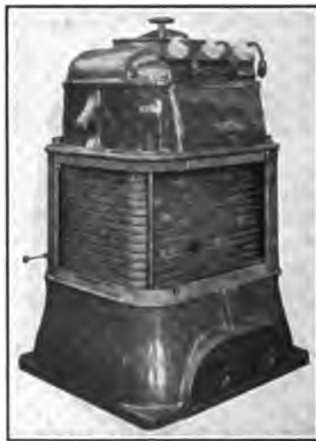
FIG. 29.—Three-phase, shell-type, 60-cycle, 330-kw., 13,200-volt primary, 430-volt secondary transformer used to investigate third harmonics
