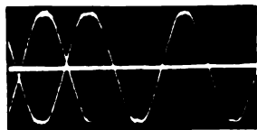
CURVE No. 138 Potential, line 2 to line 3, 460 volts.
