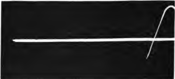
CURVE No. 175 Potential wave, neutral to line C (no load), 2,400 volts.
