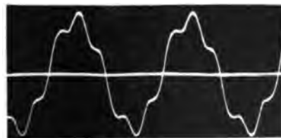
CURVE No. 109 Current in line 3, 2.0 am- peres.
