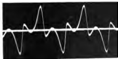
CURVE No. 128 Current in primary delta, 7.1 amperes.
