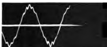
Isolated neutral, 24 poles, 530 kw., 300 rev. per min., 4150 volts. Frequency Changer CURVE No. 172 Potential wave, line to line (no load), 4083 volts.
