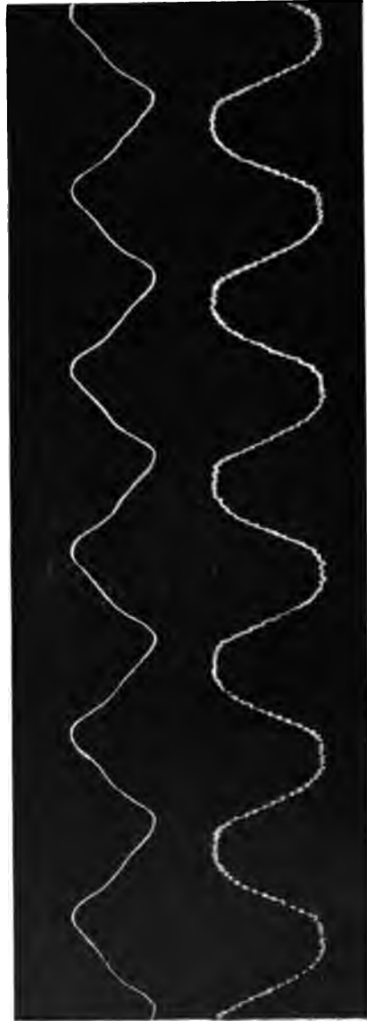
FIG. 17B—Oscillograms on single phase railway Upper curve is current taken by locomotive. Lower curve is trolley potential
