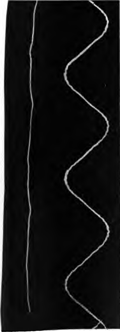
FIG. 17A—Oscillograms on single phase railway Upper curve is current...locomotive not running. Lower curve is trolley potential
