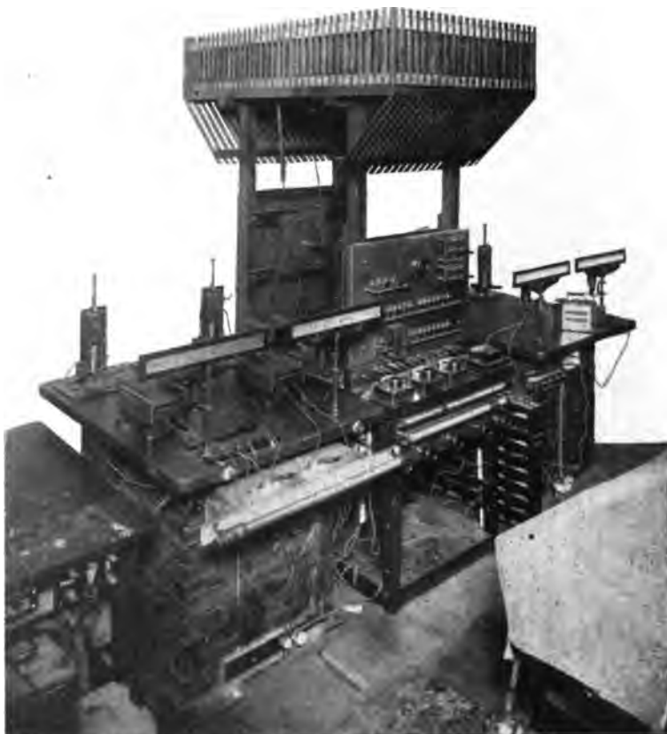
FIG. 12.—Outfit for ratio and phase angle test on potential transformers referred to in Fig. 8
