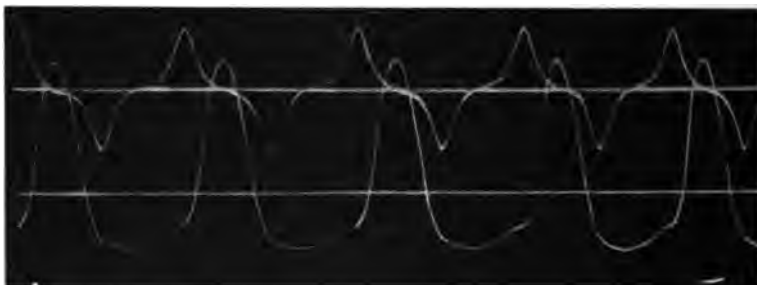
FIG. 16—Oscillogram, exciting current in 75-kw. transformer with direct current in winding. Upper curve, e.m.f. on transformer. Lower curve, exciting current
