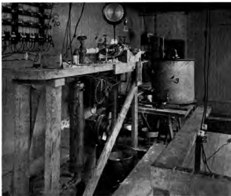
FIG. 3 SHOWING CONDENSER, ELECTRIC SUPERHEATER, VOLTAGE REGULATOR, ETC.
