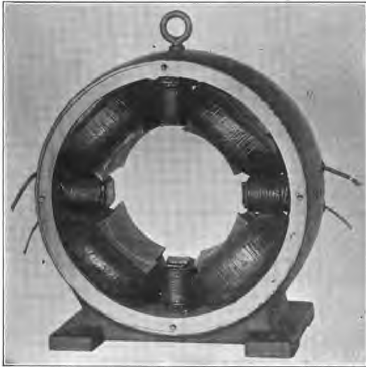
FIG. 3.—General arrangement of poles of inter-pole motor.
