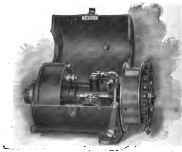
FIG. 1.—Monarch engine-stop; the device applicable to the throttle, and operated by gravity.
