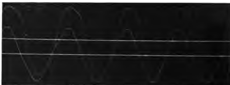
FIG. 2.—Upper curve exciting current 0.25 amp. \sqrt{\text{mean}^2} . O_1 on Fig. 1. Lower curve potential across primary. In series with trans. primary R = 10.0 and L = 0.01908 .
