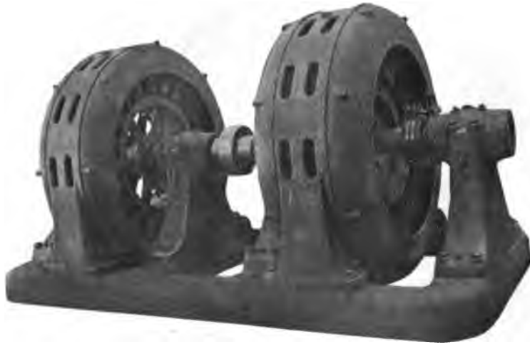
FIG. 12.—Synchronous Motor-Generator Set with Shaft Coupling. Motor, 25 cycles, 3 phase, 8 poles, 375 rev. per min.; 400-kw. Generator, 62½ cycles, 2 phase, 20 poles.
