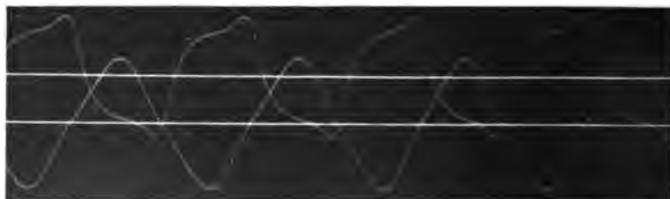
FIG. 3.—Upper curve exciting current 0.5 ampere. O_2 on Fig. 1. Lower curve potential across primary. In series with trans. primary R = 10.0 and L = 0.01908 .
