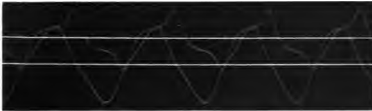
FIG. 5.—Upper curve exciting current 1 ampere. Lower curve potential across primary. In series with trans. primary R = 10 and L = 0.00164 .
