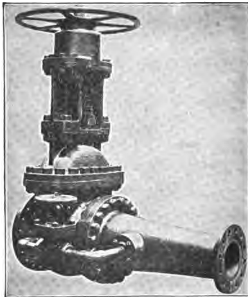
FIG. 14.—10" Roller bearing gate-valve and connections put together with forged and turned steel bolts in reamed holes for the working pressure of 1923 feet.
