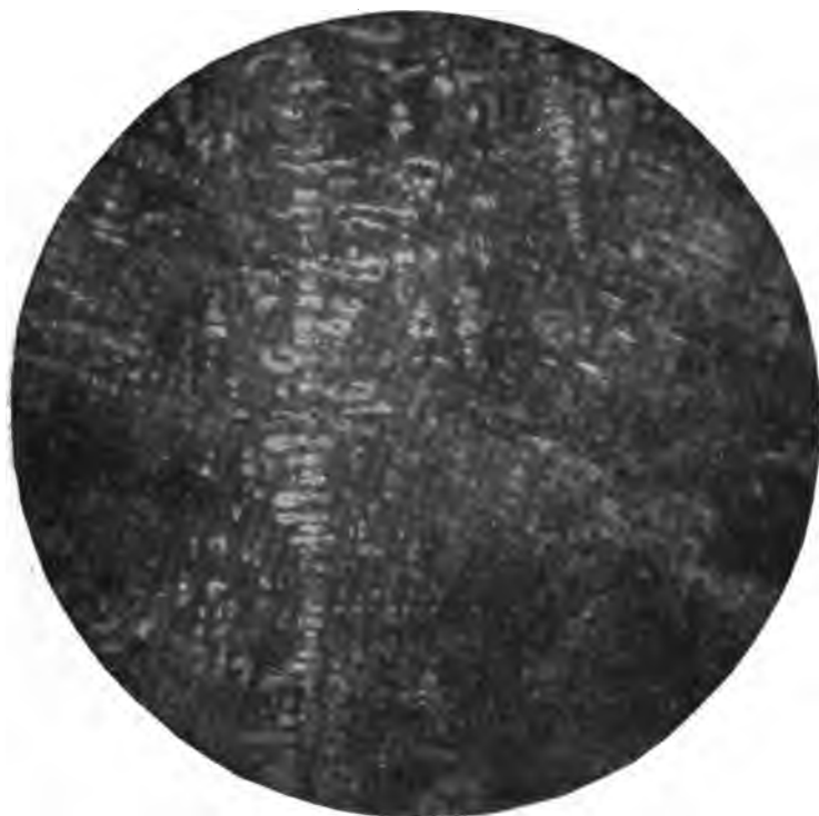
FIG. 7.—" Low " cast copper— \times 50 .
