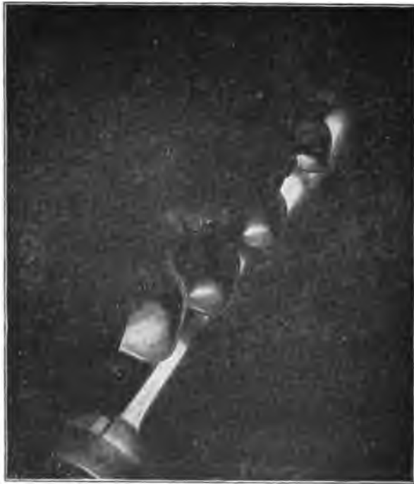
FIG. 12.—High-pressure water jet issuing from the needle-nozzle, under a head of 1923 feet.
