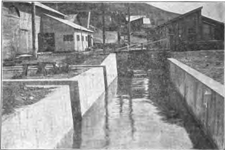
FIG. 10.—Exciter measuring weir and hook gauge measuring Apparatus. This photo also shows the still water back of the main weir.
