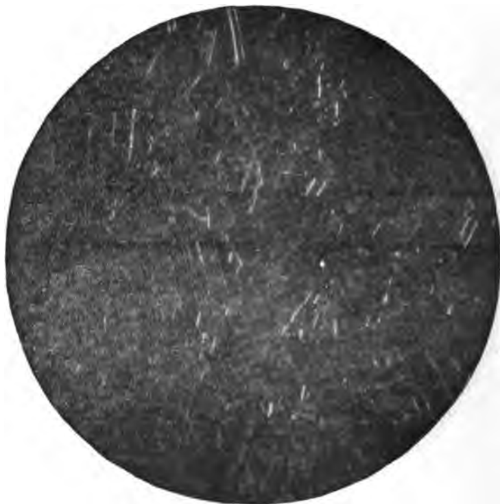
FIG. 8.—“ Burned ” trolley wire— \times 50
