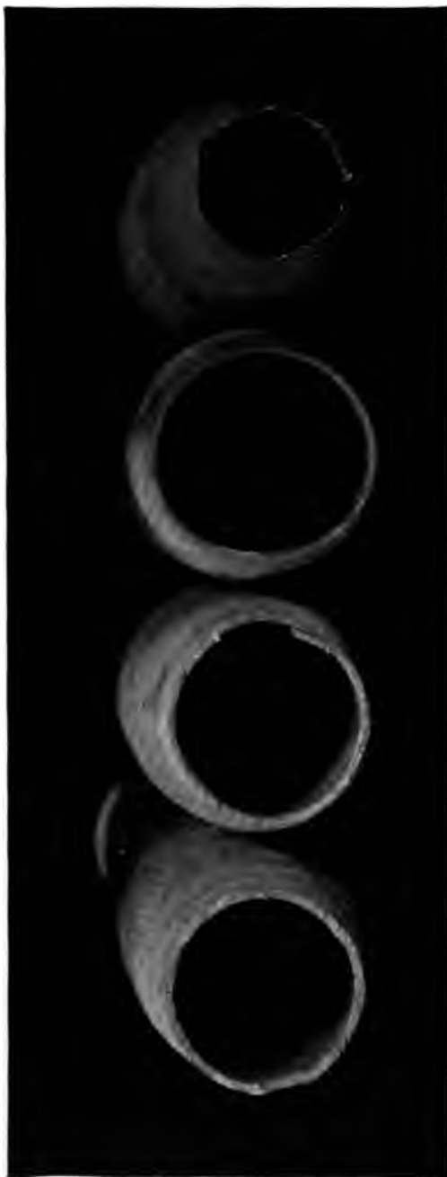
FIG. 174.—END VIEW OF FRAC- TURE, GOVT. BRASS, "A." FIG. 175.—ORDINARY BRASS, "C." FIG. 176.—SWEDISH O.-H. STEEL, "S." FIG. 177.—ALUMINUM BRONZE, Cu_{60}Al_{40} , "P."
