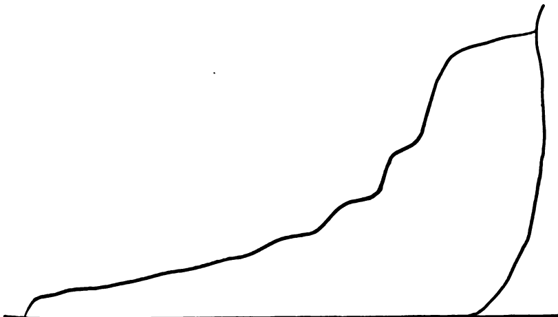
FIG. 31.—Full Power Load. 300 Revolutions. Scale 40.
