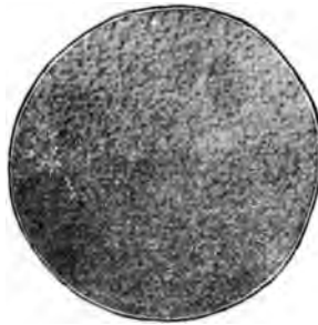
FIG. 123.—Deposit from Zinc Sulphate Solution (Acid), Magnified Five Diameters.
