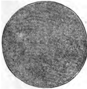
FIG. 122.—Zinc Coating Applied by Hot Galvanizing Process, Magnified Five Diameters.
