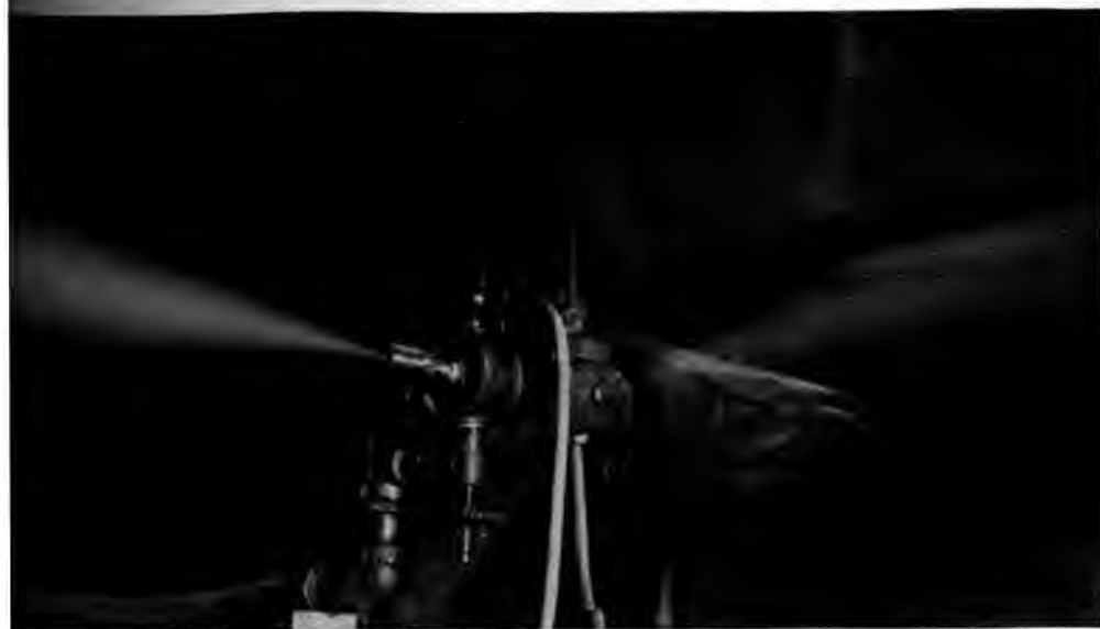
FIG. 66.—Steam at 95 Pounds Pressure Containing 1.88 per cent. Water.
