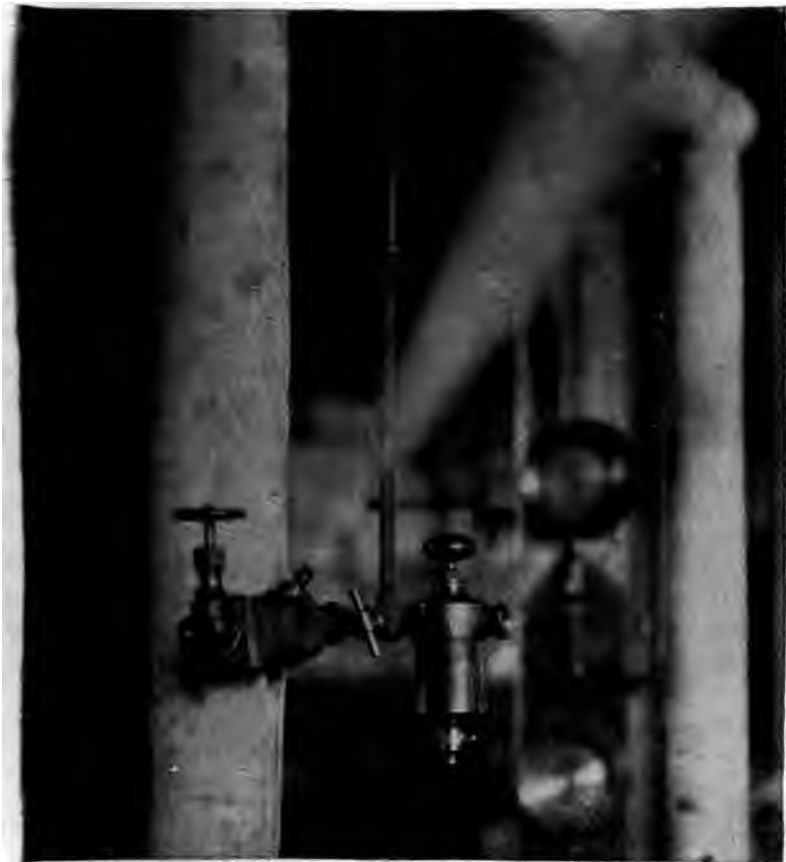
FIG. 71.—Dry Steam after Traversing 100 Feet of Covered Pipe at Velocity of 5 Feet Per Second.
