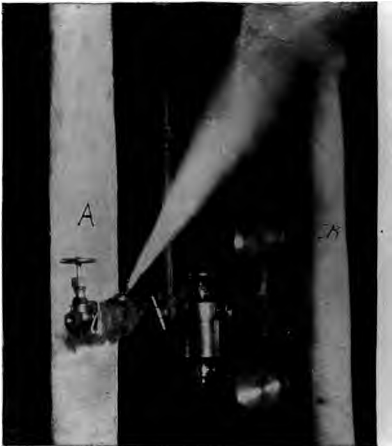
FIG. 70.—Dry Steam after Traversing 100 Feet of Covered Pipe at Velocity of 50 Feet Per Second.
