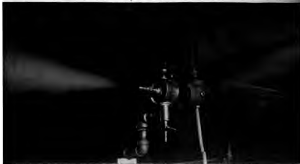
FIG. 68.—Steam at 95 Pounds Pressure, Throttled to 53 Pounds, Superheating 9 Degrees.—No Water in Condenser.
