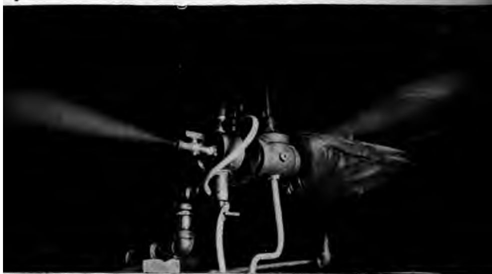
FIG. 64.—Steam at 55 Pounds Pressure Containing 1.4 per cent. Moisture.
