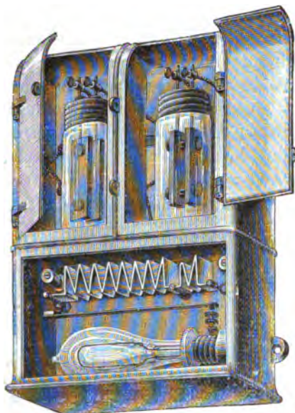
Fig. 13. Old form of two-wire Meter.
