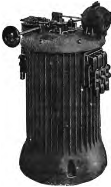
Fig. 167. Induction Potential Regulator.
