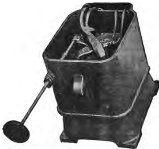
Fig. 156. Feeder Regulator with Cover Removed.
