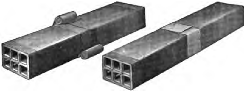
Fig. 219. Joints in Multiple-duct Conduits.
