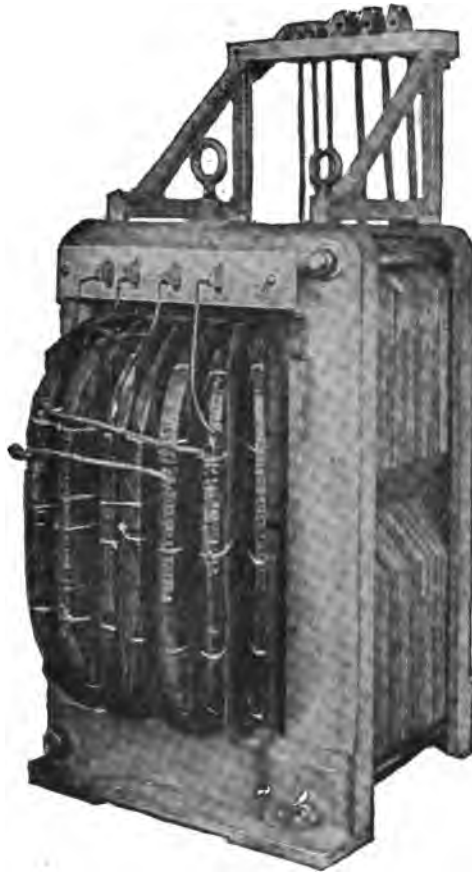
Fig. 124. Transformer with Casing Removed.
