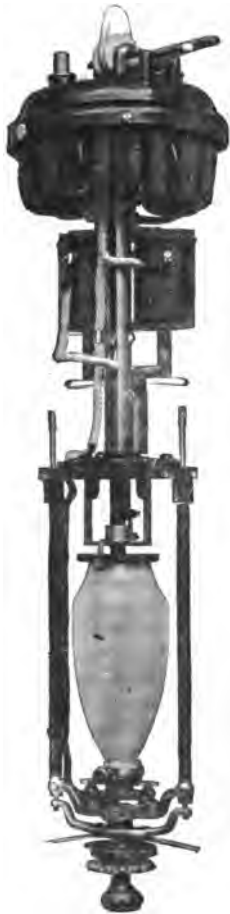
Fig. 292. Carbon-Feed, Constant Potential, Alternating Current Lamp.
