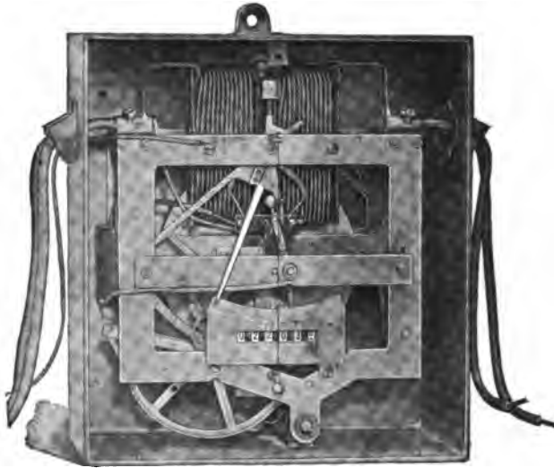
Fig. 391. The American Integrating Amperemeter.
