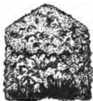
258. Appearance of Arc Light Carbons.
