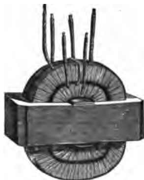
Fig. 123. Transformer with Superposed Coils.
