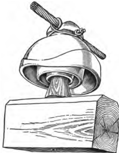
Fig. 198. The Niagara Type of Porcelain Insulator, Wood Pin and Cross-arm.
